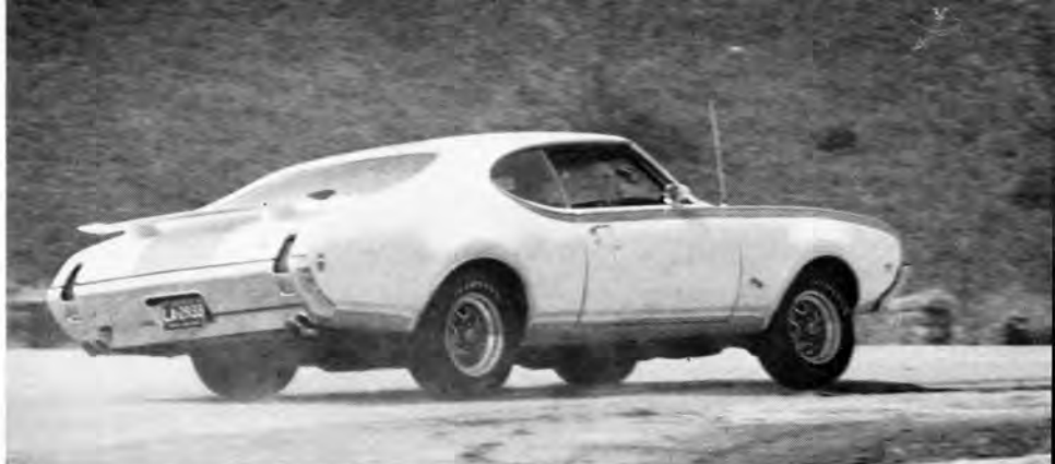
THE 455 is no heavier than 400-cid engine, and didn't spoil excellent handling of basic Olds 4-4-2. In fact, combination helped H/O make child's play of mountain roads (demonstrating slight understeer as on test circuit above).
