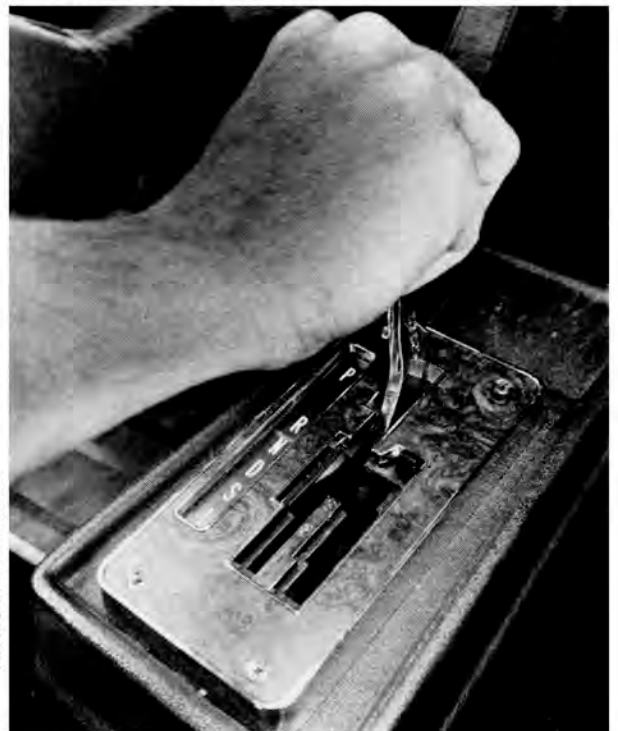
HURST Dual-Gate shifter for Turbo Hydra-Matic is drag racer's delight (and saves the transmission).
