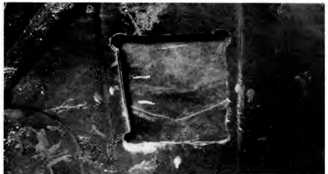
SURE ENOUGH , they just butchered a hole in original hood, then covered it with fiberglass scoops. Works, though.
