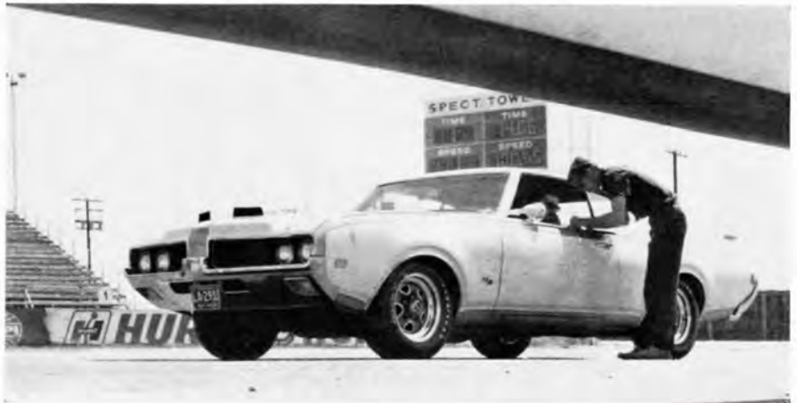
THE 455 is no heavier than 400-cid engine, and didn't spoil excellent handling of basic Olds 4-4-2. In fact, combination helped H/O make child's play of mountain roads (demonstrating slight understeer as on test circuit above).
