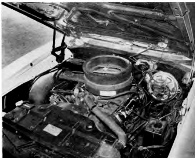
OLDS' BIGGEST , the 455-cid engine, finds way into 4-4-2 because Hurst did it. One way around GM's bhp/weight rule.
