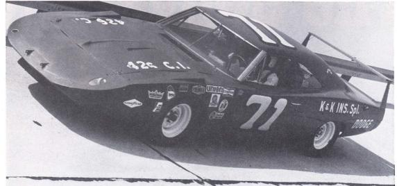
When you see the K@K Insurance Special in your rear view mirror, better step aside. Actually, Dodge put the fins on the car for the same reason they did in the late '50s - stability. Notice that the one on the race rear is manually adjustable. Hmmm.
