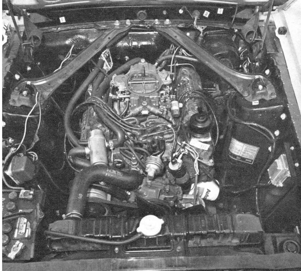
302-CID V-8 looks lost in big engine bay, but new Cleveland heads and four-barrel carburetor produce exciting Ponycar performance. It has more low end torque than competing Chevy Z/28s.
