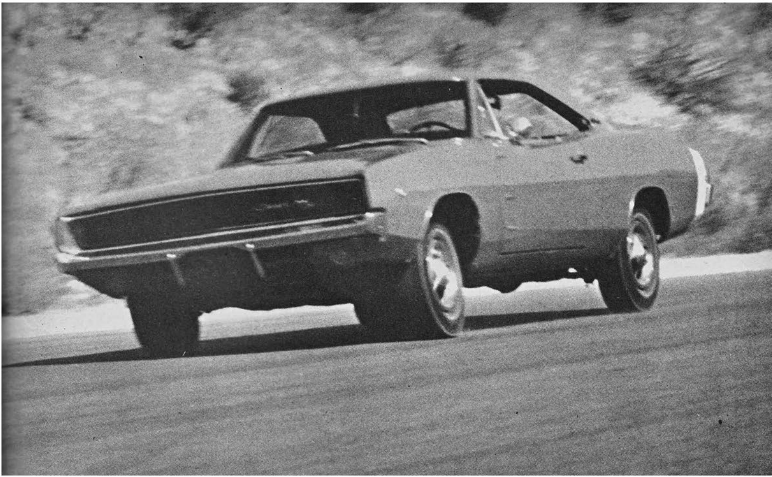
The Dodge Charger will "Garlits" out of the hole with the best of them. The big "440 Magnum" V-8 twists out a face-distorting 480 pounds of torque at 3,200 rpm. There is 375 bhp is on tap at 4,600 rpm.
