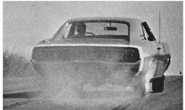
The Dodge Charger will "Garlits" out of the hole with the best of them. The big "440 Magnum" V-8 twists out a face-distorting 480 pounds of torque at 3,200 rpm. There is 375 bhp is on tap at 4,600 rpm.
