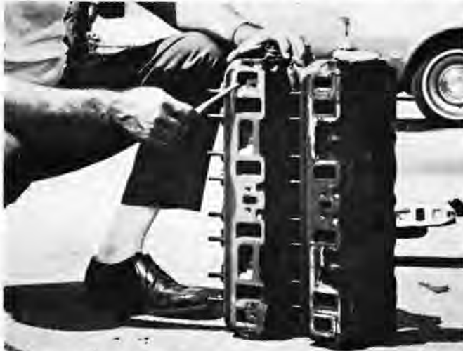
Large intake port area is readily apparent when compared to the stock 289 unit. 351 head gaskets are a must for sealing.
