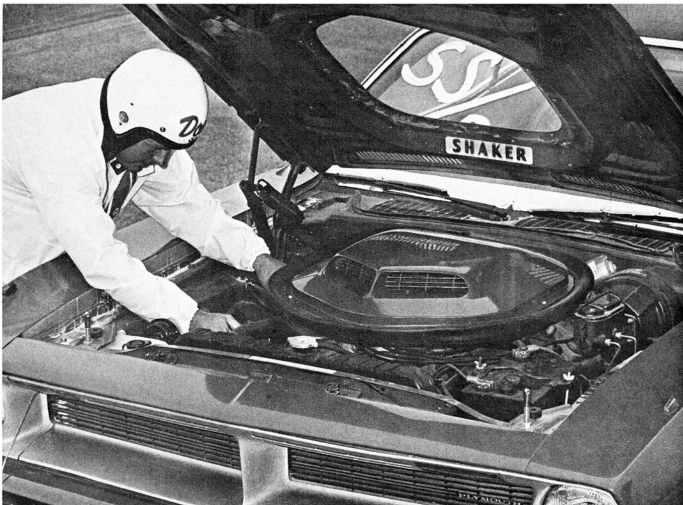
Drag team star Don Grotheer gives hemi engine the once over before starting our tests. Hemi has hydraulic lifters for '70, but performance is not affected by the change.
