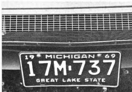
Small mesh grille and custom duct work keep the mill at normal running temperature. Hood is actually secured only by chromed NASCAR hood pins. Flush key locks are recommended.
