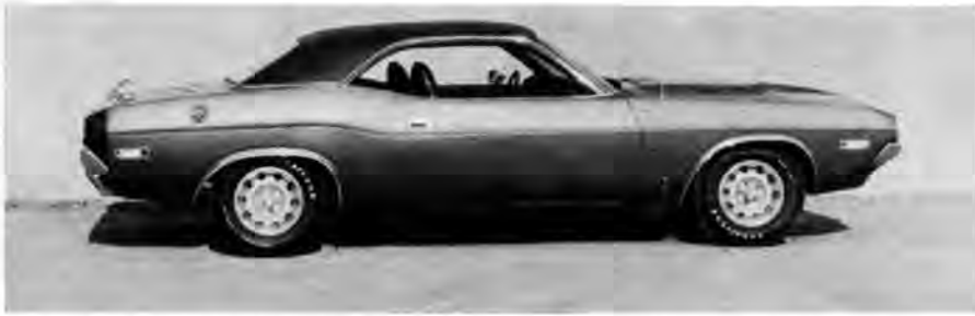
TOP—Flush door grips, smooth windshield angle and moldings, and slippery shaped front end all contribute to low wind noise. Wheel spider caps bolt on from back. BELOW, LEFT — The back seat could be larger; if any smaller, it would no longer fit the description. RIGHT — Trunk is for bachelors who travel only by airplane.
