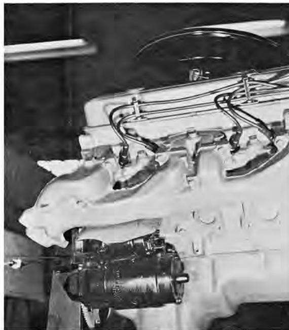
BELOW LEFT —The latest head castings for the '70's (top) have a fully machined area around the intake valve and more breathing room around the exhaust than the heads used on the old 400 engine. BELOW RIGHT —Even the stock GS 455 exhaust manifold is quite free-flowing, but the best results come in the form of headers with 2½ inch pipes and stacks of 36 to 40 inch length. If you do keep the cast jobs, you can remove the exhaust stoves and then tape up the air cleaner to make the best use of the cool air supply.
