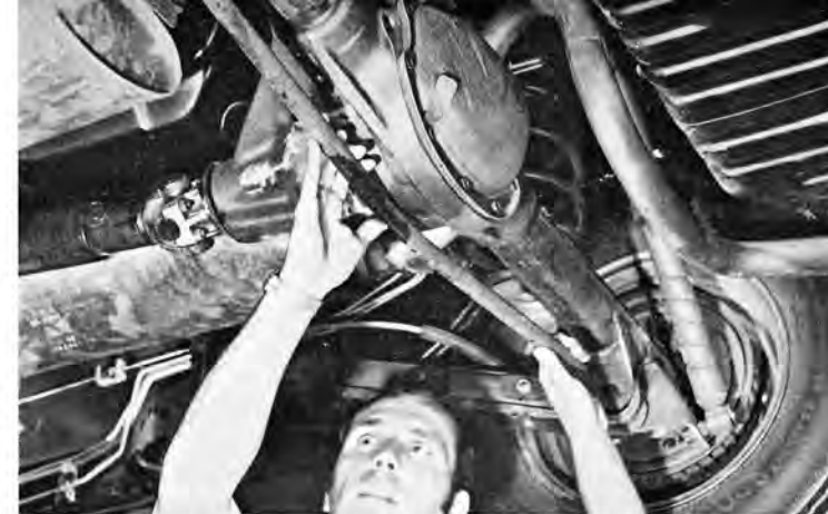
ABOVE—The new stabilizer bar at the rear, plus the added control in the shocks brings remarkable handling improvement. Gears range from 3.64 to 4.33.
