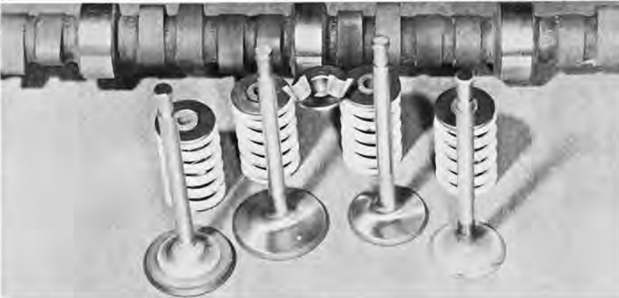
ABOVE—The new intake valves (center left) have a flatter swirl-polished undersection. They measure 2 1 / 8 ". The exhausts are big, too, and total 1 3 / 4 ". BELOW—In the new heads, the oil is metered to the rocker arms by the lifters and the pushrods. A Stage II camshaft is available with #1385557. Better use it for strip only, though.
