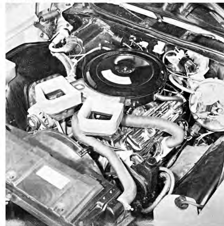
ABOVE—When you are souping the GS 455, use the richer metering rods, part number 7034822 and add a separate fuel filter to replace the one that's in the carburetor. BELOW—This monumental air cleaner has two snorkels which attach to the hood, plus vacuum operated valves that control hot air coming up from the exhaust manifold "stoves." The plastic reservoir at the extreme left is new and for filling the radiator. Saves burned flesh.
