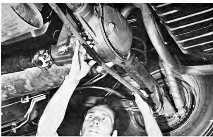
ABOVE —The new stabilizer bar at the rear, plus the added control in the shocks brings remarkable handling improvement. Gears range from 3.64 to 4.33.
