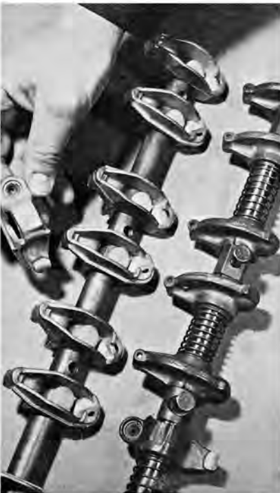
BELOW LEFT—The old forged rocker arms, together with all the springs and spacers, have been replaced with new "bath-tub" type rockers which are located by nylon bushings. The new rocker shaft is nitrided for surface harness. These new valve train parts allow engine revs to 6200 with the Stage II stuff. Good, eh? BELOW RIGHT—A Buick technician shows off the new big block. Its big bore and stroke ratio allows more room around the valves and thus better breathing characteristics.
