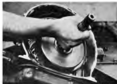
ABOVE—Pull out the input shaft and forward clutch drum, but leave the direct clutch drum. Remove thrust washer from the former. BELOW—Brass or wooden drift is used to knock out input shaft from the forward clutch drum.
