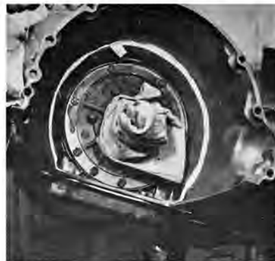
ABOVE—Cut bell housing on Turbo case with shaft and pump seal covered so no filings get into the transmission.
