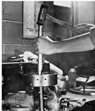
ABOVE—Pull out the input shaft and forward clutch drum, but leave the direct clutch drum. Remove thrust washer from the former. BELOW—Brass or wooden drift is used to knock out input shaft from the forward clutch drum.
