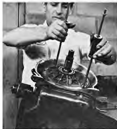
ABOVE—Pull front pump out with slide hammers. If there is a wire attached to the pump, cut it (variable pitch units only). Tape the wire and tuck it to one side so it won't hit or rub on moving parts.
