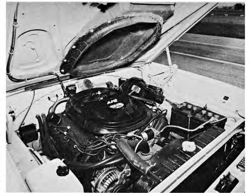
ABOVE—The hemi is still boss! Though it has been relegated a hydraulic lifter cam, to help with emission control, the specs are still the same and the performance may be even better. It sounds just as wild as the previous numbers—just a better deal all the way 'round. The filterless air cleaner base makes an excellent air-router, especially with the trap door ajar.
