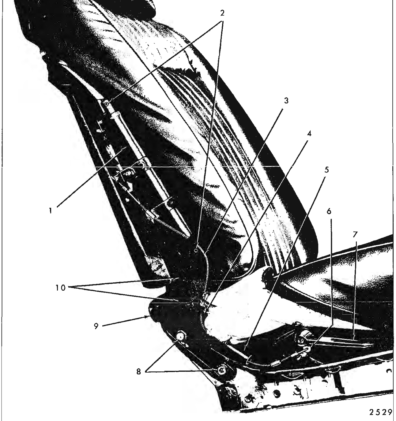
Fig. 15-56--Reclining Seat Back and Positioning Unit
