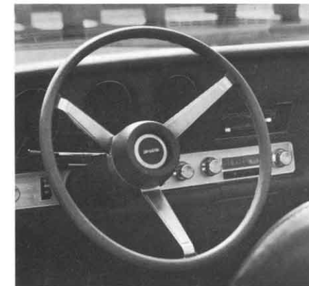
Custom Sports Steering Wheel (Code 462—UPC N34). One style available for all models. New shallow design and new molded vinyl hub with center horn button ornament. It has a smart, simulated wood appearance and three, equally spaced, bright steel spokes. (F)
