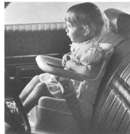
Child Safety Seat. Available all models. Provides extra protection for small child. Utilizes standard seat belt. Sturdily constructed with special chest retainer strap to restrict forward movement during quick stops. Ivory color only. (D)
