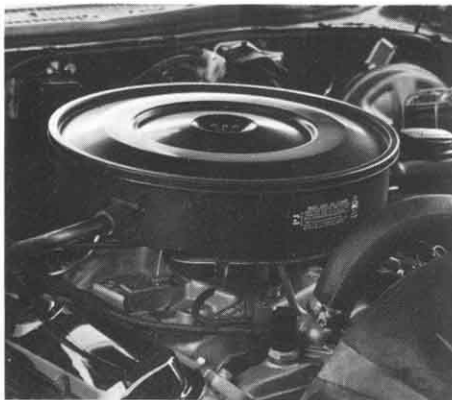
Dual-stage, Heavy-duty Air Cleaner (Code 731—UPC K45). Dual-filter design consists of wetted paper in filter, surrounded by polyglycol wetted polyurethane foam outer filter. Fine filtration, extended surface. Available all models except those equipped with 428 H.O. engines. (F)
