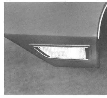
Cornering Lamps (Code 651—UPC T87). Available for all models except Firebird. Part of Lamp Group (Code 332). Lights up blind spots when turning. Goes on when headlamps are on and turn signal is activated. Mounted on forward side of front fender. (F)
