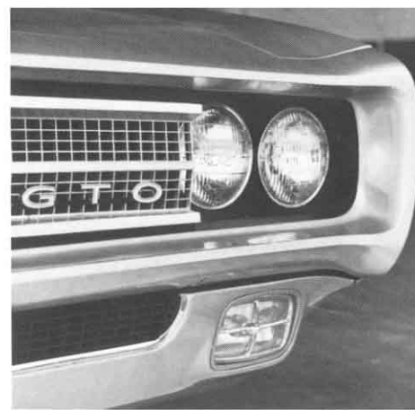
Concealed Headlamps (Code 414—UPC T83). Available only for GTO models. Give a clean, unbroken appearance to the front end. Sections of the grille swing down and
