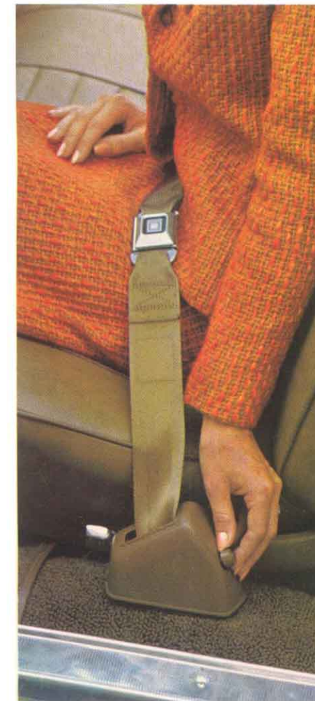
Custom Seat Belts and Front Shoulder Belts (Code 431—UPC WS1). Features new, compact, press-to-release pushbutton buckle on a fixed-length belt for driver and outboard passenger. Belt adjustment is made after belt hook-up by moving belt toward outboard retractor. This permits the automatic locking retractor to take up slack and provide desired tension. New twist button on retractor housing releases belt tension to permit wearer to move away from position without disconnecting buckle. All belts, front and rear, available in seven harmonizing colors. Available for all models except Firebird. Also available are Custom Seat Belts and Front and Rear Shoulder Belts (Code 432—UPC WS2). (F)
