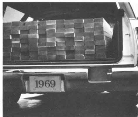
Superlift Shock Absorbers with Automatic Level Control (Code 544—UPC G67). Adjustable air springs built into rear shock absorbers maintain level ride, even with heavy trunk or trailer tongue loads. Vacuum-operated air compressor in engine compartment automatically keeps the rear of
