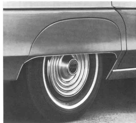
Fender Skirts (Code 674—UPC T58). Optional at extra cost for Catalina and Executive models except station wagons. Give smooth continuous lines to body sculpturing. (Standard on Bonneville.) (F,D)
