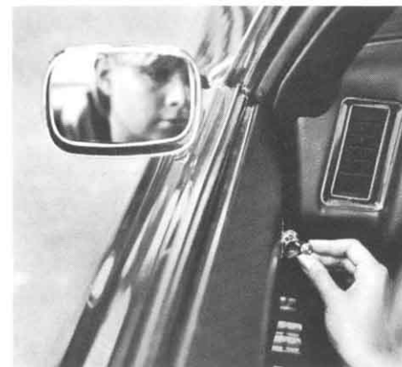
Remote-control Outside LH Mirror (Code 424—UPC D33). Mounts on left-hand door. Adjusted from convenient controls inside car. Available all models. (F,D)
