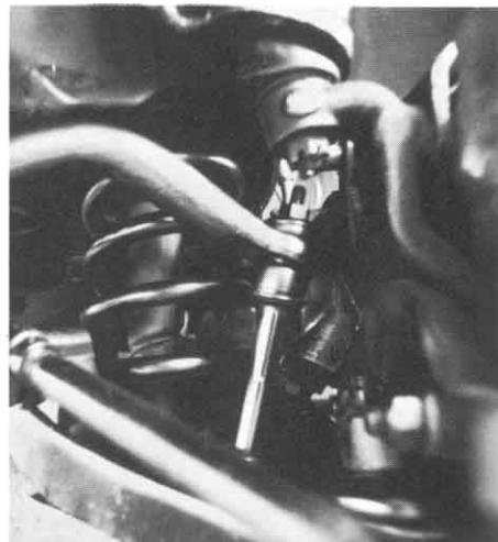
Heavy-duty Shocks and Springs (Code 622—UPC F40). Maintain proper trim and give better control. Especially helpful when heavy loads are carried in car trunk. Available all models, except Firebird. (F,D)
