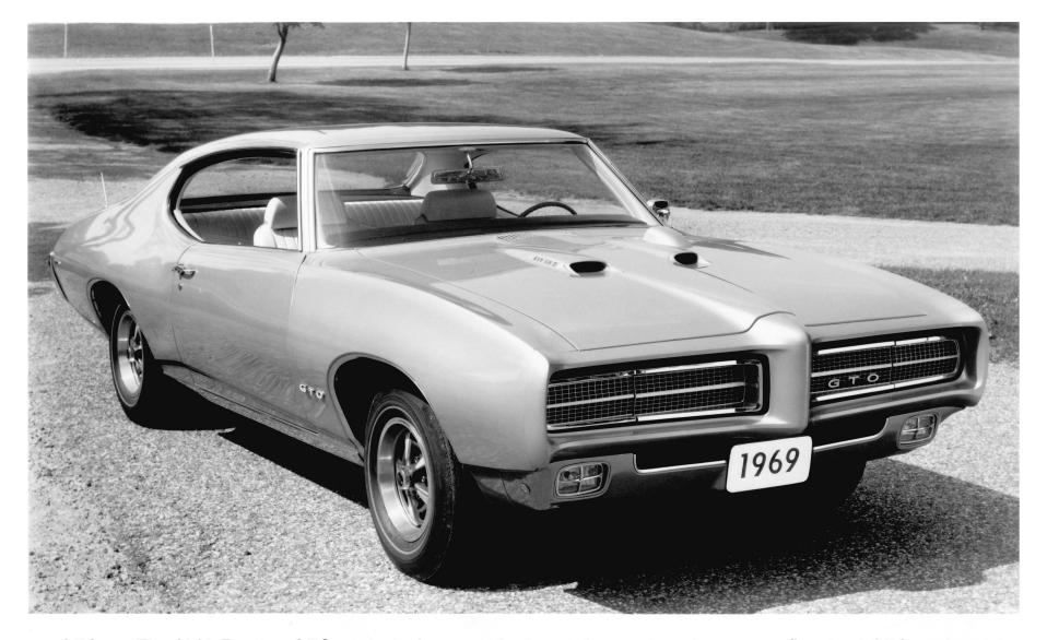
GTO -- The 1969 Pontiac GTO again features exclusive styling and performance. Standard GTO equipment includes a 400 cubic-inch V-8 engine, Endura front bumper and wide oval tires. Concealed headlamps, hood mounted tachometer and two Ram Air packages head a long list of popular options. The GTO is offered in a convertible and two-door hardtop coupe.
