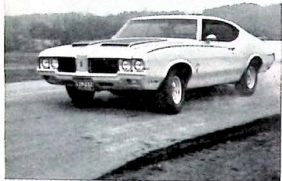
High spring rates, anti-roll bars front and rear, wide rubber make Rallye 350 a real handler. Rear deck spoiler is adapted from defunct Hurst-Olds.
