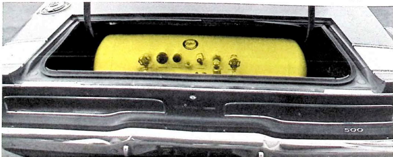
Each carburetor has its own fuel delivery system, requiring use of two solenoid lock-off valves (far left), which permit flow only when ignition is on. Induction system uses base assembly from fuel injection unit (left) and 900-cubic-inch plenum box. Excess flow sensing valves in 23-gallon tank automatically shut should a fuel line rupture, two of several safety devices.
