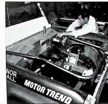
Front roll cage cuts bovine damage. The Broncos are rebuilt from the frame up.
