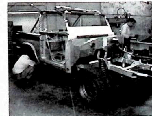
Once chassis is on wheels, roll cage can be built and basic body shell bolted on. Complete car weighs 3700 pounds and has speed of 122.
