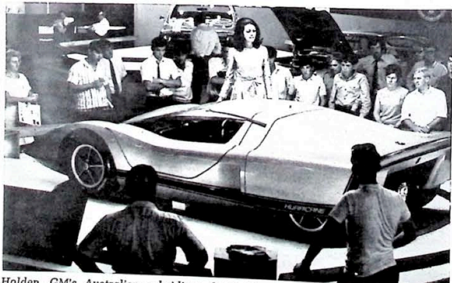
Holden, GM's Australian subsidiary, built this dream car, the Hurricane. The fiberglass-bodied car has a 260-hp V8, oil-cooled disc brakes and TV rear vision.
