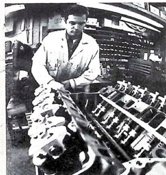
Aluminum rocker arms are installed in stock block at Traco shop.
