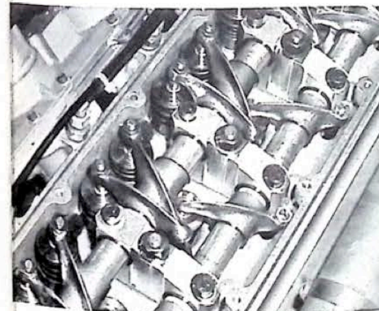
Pumping out 606 hp at 8500 rpm on gasoline, the engine ran into heating problems in early track tests. These have been corrected and spectacular results are expected in the near future. Relatively low lift, short duration camshaft speaks to intake valves with forked rocker arms. Ends of clearance adjusting screws are articulated for better geometry.
