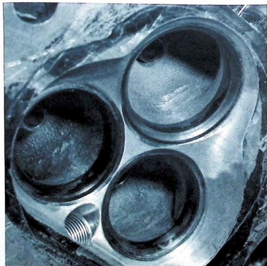
Grass-roots presidential candidate Dan Gurney is still active in refining the small block Ford for racing. Latest development is a twin intake valve variation of the famed Gurney-Weslake head. Flow has been improved by about 100 cfm on the intake side and 80 cfm on the exhaust, resulting in a more than 60 hp gain. All valves use 45-degree, .030-inch seats.
