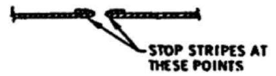
SECTION "B-B" (TYPICAL AT EDGES OF DOOR, FRONT FENDERS AND REAR QUARTER PANEL)
