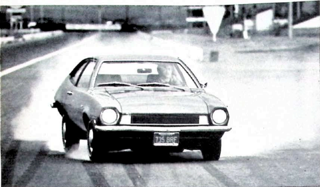
Left: Pinto's rack and pinion steering, handling, and 4-speed make it supreme fun to drive; Pinto owners even wave to each other. Rear brakes tend to lock in panic stop, however, resulting in sharp pull to the left. Above: Fit and finish of interior is on a very high level, but seats lack comfort for long trips. Car shown has the optional 3-speed automatic, requiring 2-liter engine; both standard equipment. Though not powered, ventilation is good.
