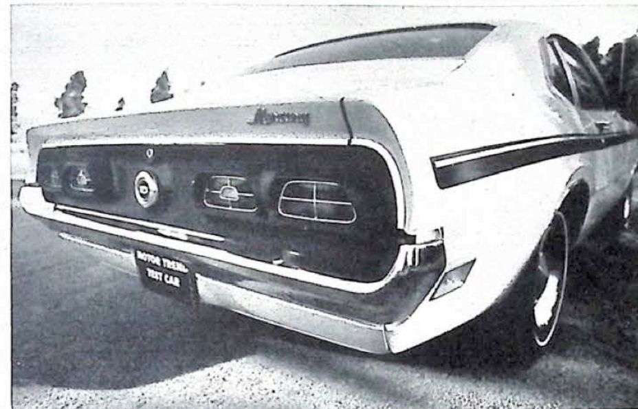
Above: Mercury displayed shrewd planning by utilizing many existing parts to convert Maverick into latest Comet. Taillights, hood scoop, and center grille section all come from Cyclones. Below: Nova is unchanged from moderately popular '70 version, with exception of such trim details as clear back-up lights and new bezels for headlights. Interior quality ranked highest.
