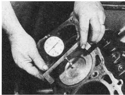
Brady made his own deck height checking stand.
