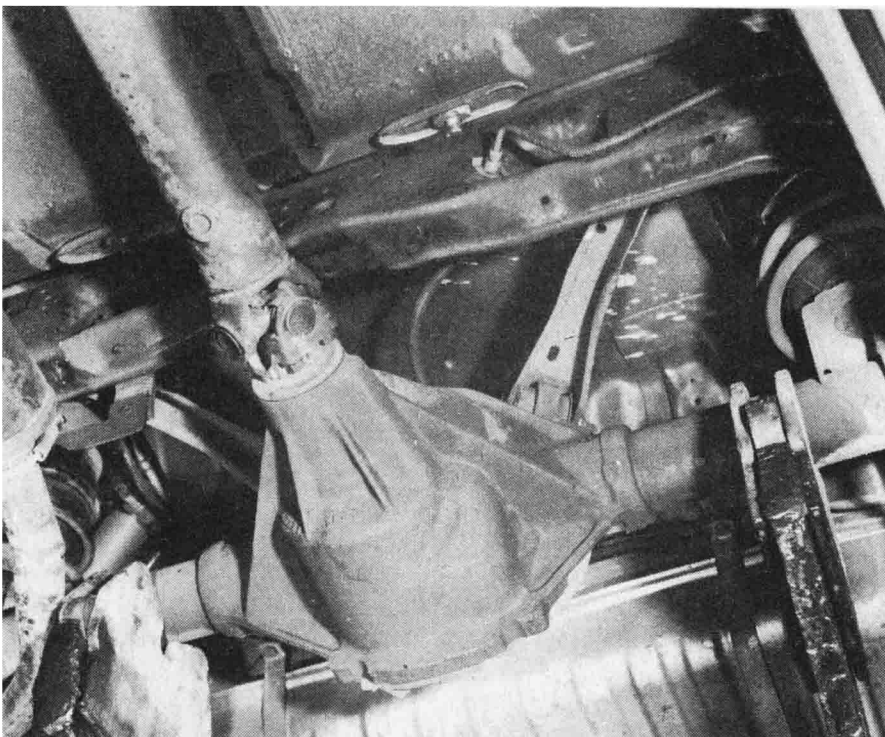
Aluminum cover increases Olds rear's capacity. Canadian Chevy rear uses 5.38's!
