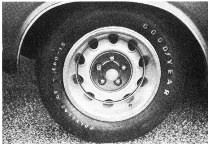
E60-15 Polyglas skins are eight inches across; they excel in the traction department when mounted on seven-inch Rally wheels.
