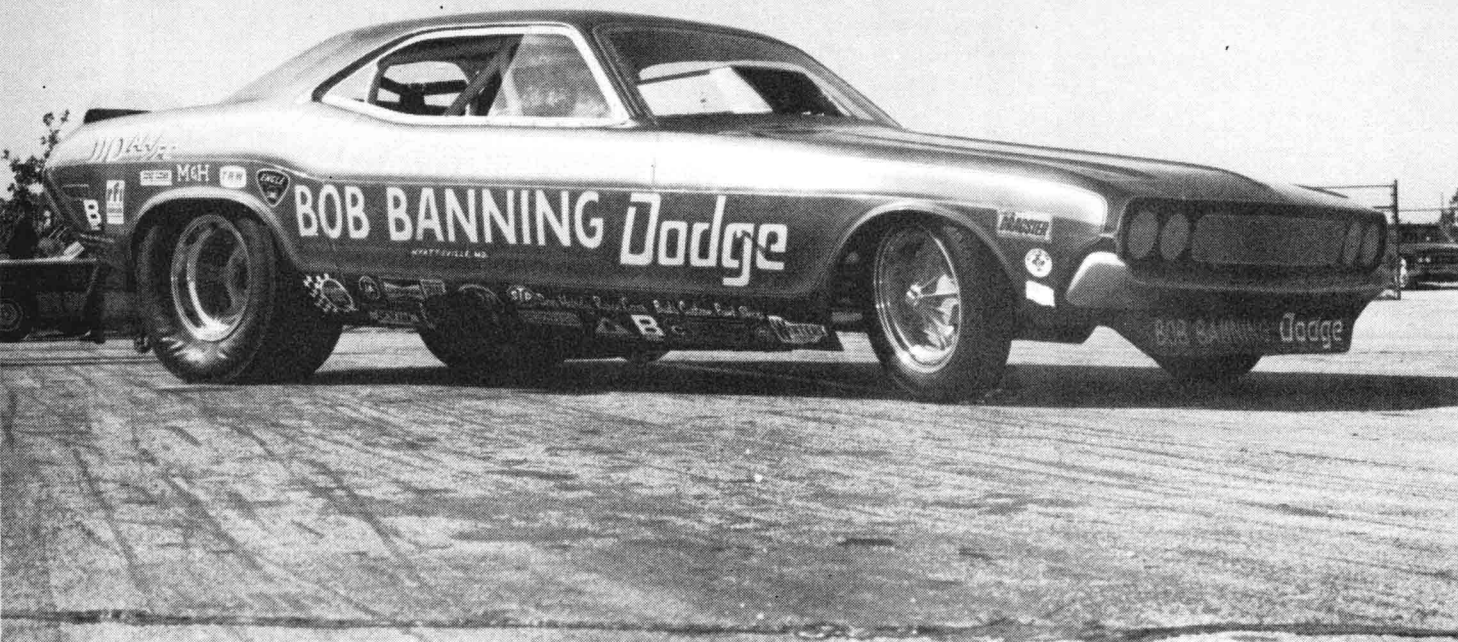
Ace chassis builder, Don Hardy fabricated the entire 118-inch chassis and the tubular front axle. Tom Sneden pilots "Banning's Boiler."
