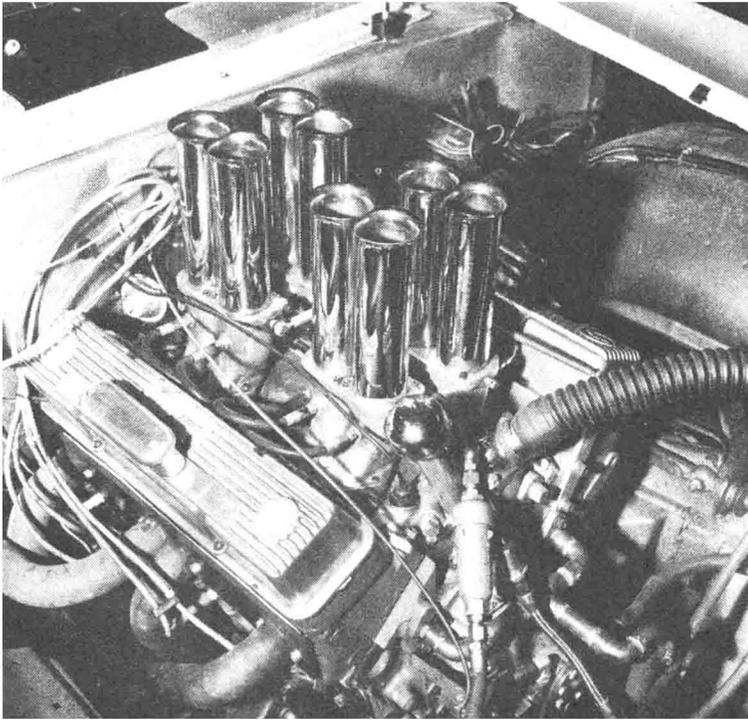
Eight-inch stacks will yield to six-inchers for 8200 rpm trips.
