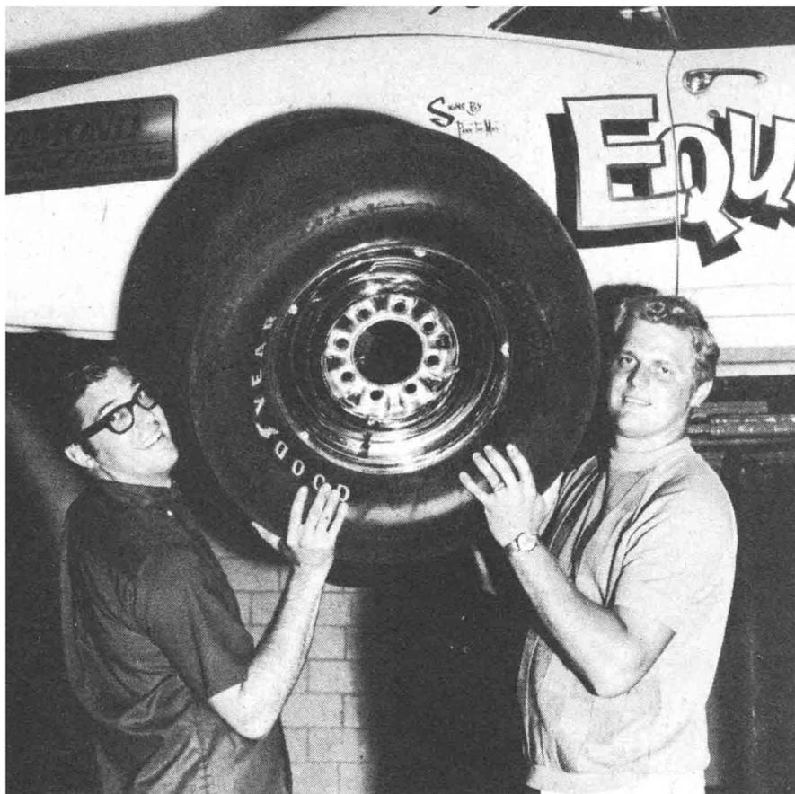
The 15X7 wheels had to be home made. Truck center is pressed into Corvette outer rim.
