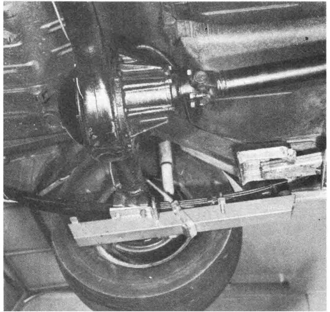
Full torque is harnessed by always having full T-bar/spring contact.
