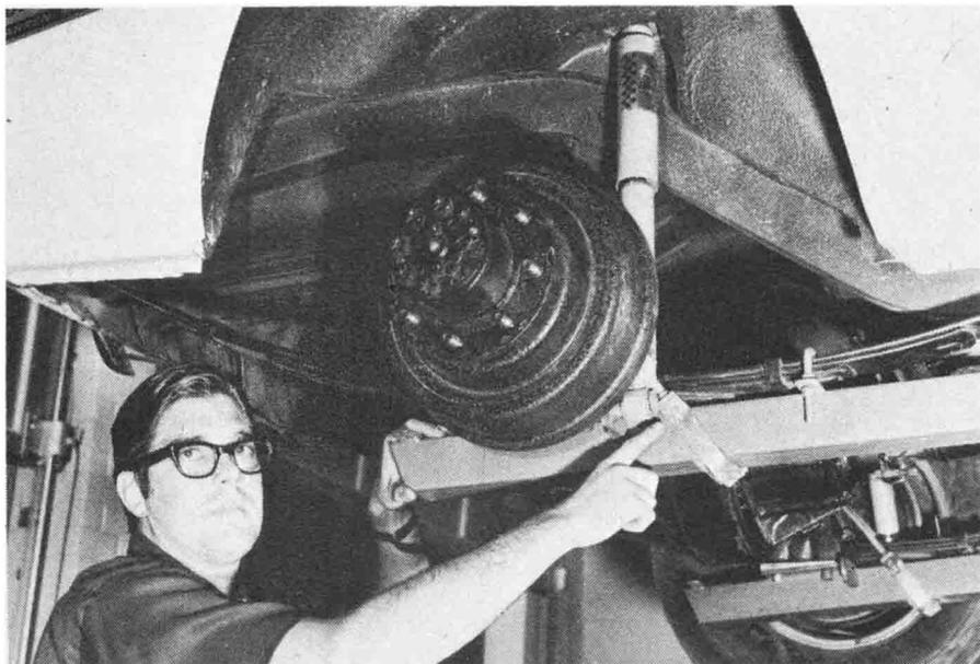
Truck rear features built-in safety hubs with Timken roller bearings. Brakes are light.
