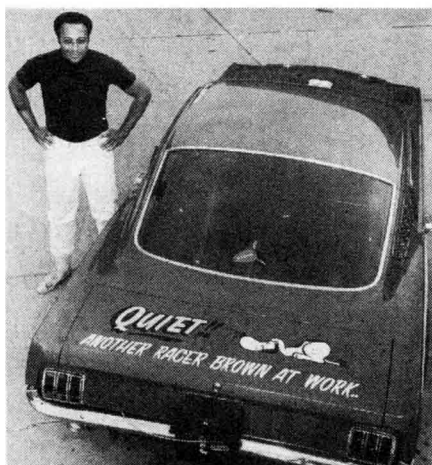
C/Gasser weighs 2540 pounds of which 1340 is at rear and 1200 pounds at the front.
