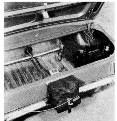
Aluminum panel replaces steel section between trunk and body. Chute riser line mounts inboard.
