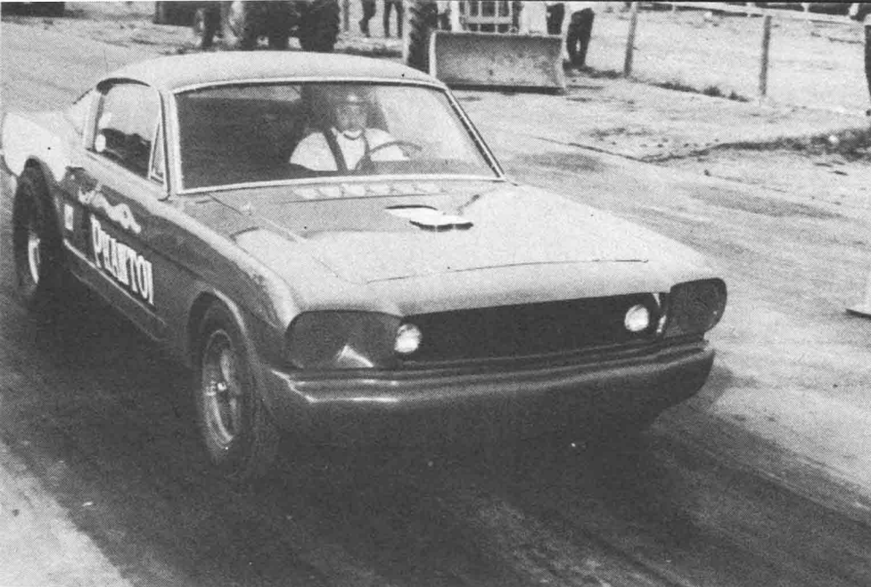
Glass front is masked for minimum air entry. All steel, including spring towers, was removed.
