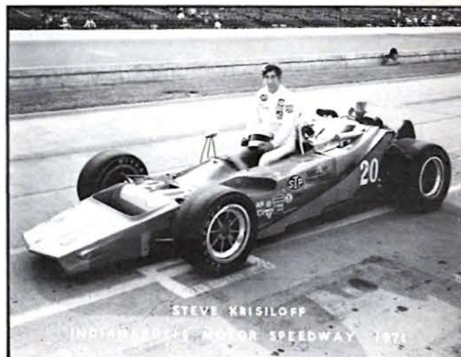
Car No.: 20 Driver: Steve Krisiloff (STP Gasoline Treatment Spl.) Qual. Speed: 169.835 Day: 3 Start: 27th Finish: 31st Entrant: STP Corp. Chief Mechanic: Vince Granatelli Engine: Ford Turbo Plugs: Autolite Tires: Firestone Front size: 4.75-12.40 x 15 (154) Rear size: 5.30-17.00 x 15 (154) Chassis: McNamara Engineering features: Early version car No. 5 with front spoiler mounts still in place Driver's previous finishes: Rookie (passed test 1970) History of car (Year, driver, qual.speed, start, finish, etc.): New Car Money won: $13,260 Laps completed: 10 (oil leak; wrecked in third turn on lap 10)
