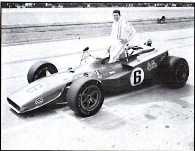
Car No.: 6 Driver: Roger McCluskey (Sprite Spl.) Qual. Speed: 171.241 Day: 3 Start: 22nd Finish: 9th Entrant: Lindsey Hopkins Chief Mechanic: Don Kenyon Engine: Ford Turbo Plugs: Champion Tires: Goodyear Front size: 10.40 x 15 Rear size: 15.70 x 15 Chassis: Kuzma-Kenyon Engineering features: Re-located oil tank—wedge type design Driver's previous finishes: 27th '61; 16th '62; 15th '63; 30th '65; 13th '66; 19th '67; 29th '68; 14th '69; 25th '70* History of car (Year, driver, qual.speed, start, finish, etc.): 1970 back up car not run Money won: $22,980 Laps completed: 188 (running) *Also relieved Mel Kenyon for 16th
