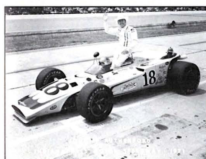
Car No.: 18 Driver: Johnny Rutherford (Patrick Petroleum Spl.) Qual. Speed: 171.151 Day: 3 Start: 24th Finish: 18th Entrant: Michner Petroleum, Inc. Chief Mechanic: Mike Devin Engine: Offenhauser Turbo Plugs: Champion Tires: Goodyear Front size: 10.40 x 15 Rear size: 15.70 x 15 Chassis: 1967 Eagle Engineering features: Wedge type body Driver's previous finishes: 29th '63; 27th '64; 31st '65; 25th '67; 18th '68; 29th '69; 18th '70 History of car (Year, driver, qual.speed, start, finish, etc.): 1967 Jerry Grant bumped; 1968 Jerry Titus too slow; 1969 Johnny Rutherford 166.628 17-29 (lap 24 hole in oil tank); 1970 Johnny Rutherford 170.213 2-18 (lap 135 broken header) Money won: $16,682 Laps completed: 128 (running, had moved from 24th to 7th before ignition problems)
