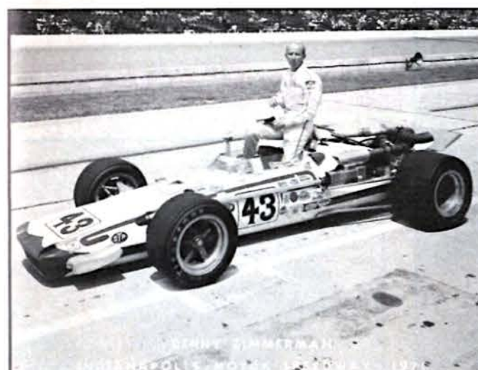
Car No.: 43 Driver: Denny Zimmerman (Fiore Racing Enterprises Spl.) Qual. Speed: 169.755 Day: 3 Start: 28th Finish: 8th Entrant: Fiore Racing Ent. (F.J. Fiore) Chief Mechanic: J. Wadsworth Engine: Offenhauser Turbo Plugs: Champion Tires: Firestone Front size: 4.75-12.50 x 15 (154) Rear size: 5.30-17.00 x 15 (154) Chassis: Vollstedt Design based on: Lotus Driver's previous finishes: Rookie (passed test 1969) History of car (Year, driver, qual.speed, start, finish, etc.): 1966 Billy Foster 159.490 12-24 (wrecked); 1967 Lucien Bianchi 162.484 bumped; 1968 Jim Malloy 165.032 14-22 (lap 64 engine trouble); 1969 Jim Malloy 167.092 13-11 (lap 165 flagged); 1970 not entered Money won: $26,658 Laps completed: 189 (running). ROOKIE-OF-THE-YEAR.
