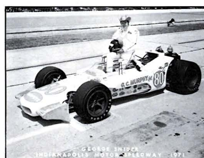
Car No.: 80 Driver: George Snider (G.C. Murphy Spl.) Qual. Speed: 171.600 Day: 3 Start: 21st Finish: 33rd Entrant: Leader Cards, Inc. Chief Mechanic: A.J. Watson Engine: Ford Turbo Plugs: Autolite Tires: Firestone Front size: 4.75-12.50-15 (20) Rear size: 6.25-17.00-15 (20) Chassis: 1968 Eagle Design based on: Monocoque principle Engineering features: Modified rear suspension—open wedge bodywork Driver's previous finishes: 21st '65; 19th '66; 26th '67*; 31st '68; 16th '69; 20th '70 History of car (Year, driver, qual.speed, start, finish, etc.): 1968 Bobby Unser 169.507 3-1 (200 laps at 152.882 mph); 1969 not at track; 1970 Mike Mosley 166.651 12-21 (lap 96 cracked block) Money won: $13,974 Laps completed: 6 (stalled on front straight) *Relieved by Lloyd Ruby
