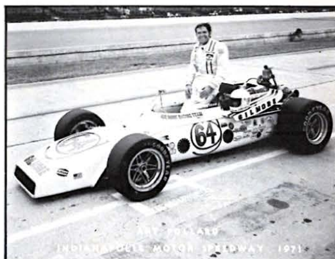
Car No.: 64 Driver: Art Pollard (Gilmore Racing Team) Qual. Speed: 169.500 Day: 4 Start: 31st Finish: 26th Entrant: Gilmore Champ. Racing, Inc. Chief Mechanic: C. Brawner Engine: Ford Turbo Charged Plugs: Autolite Tires: Goodyear Front size: 10.40 x 15 Rear size: 15.70 x 15 Chassis: Brawner Scorpion Design based on: Brawner Hawk (Brabham) Driver's previous finishes: 8th '67; 13th '68; 31st '69; 30th '70 History of car (Year, driver, qual.speed, start, finish, etc.): 1970 Roger McCluskey 169.213 4-25 (lap 62 Split crankcase weld) Money won: $14,770 Laps completed: 45 (dropped valve)
