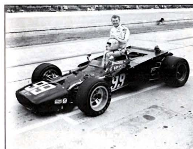
Car No.: 99 Driver: Bob Harkey (Joe Hunt Magneto Spl.) Qual. Speed: 169.197 Day: 4 Start: 32nd Finish: 22nd Entrant: Joe Hunt Chief Mechanic: Joe Hunt Engine: Offenhauser Turbo Plugs: Champion Tires: Firestone Front size: 4.75-12.50 x 15 (154) Rear size: 5.30-17.00 x 15 (154) Chassis: Gerhardt Engineering features: Modified wedge bodywork Driver's previous finishes: 8th '64 History of car (Year, driver, qual.-speed, start, finish, etc.): 1969 Mel Kenyon 165.426 24-4 (200 laps at 152.177); 1970 Denny Zimmerman, too slow Money won: $15,399 Laps completed: 77 (rear end failure)
