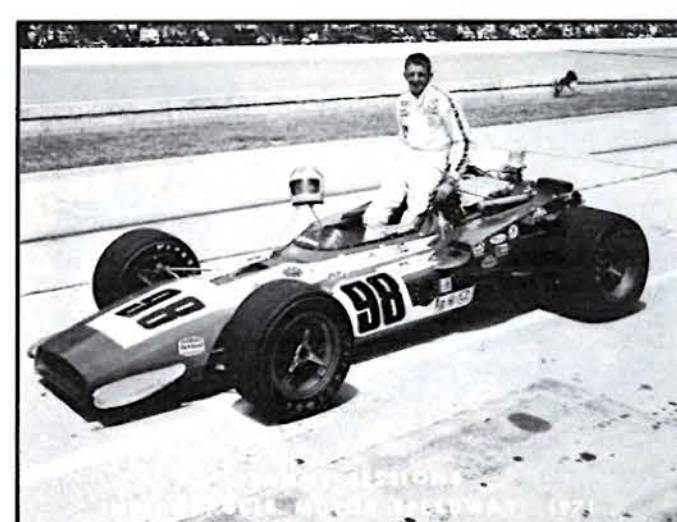
Car No.: 98 Driver: Sam Sessions (Wynn's Kwik Kool Spl.) Qual. Speed: 170.358 Day: 3 Start: 25th Finish: 27th Entrant: Agajanian-Faas Racers, Inc. Chief Mechanic: Leonard Faas Sr. Engine: Ford Turbo Plugs: Champion Tires: Firestone Front size: 4.75-12.50 x 15 (20) Rear size: 6.25-17.00 x 15 (20) Chassis: '70 P.J. Colt Design based on: Lola Driver's previous finishes: 9th '68; 12th '69; 12th '70 History of car (Year, driver, qual.speed, start, finish, etc.): 1968 Al Unser wrecked in practice; 1969 Bud Tingelstad 166.597 18-15 (lap 155 valve failure); 1970 not entered Money won: $13,721 Laps completed: 43 (broken valve)
