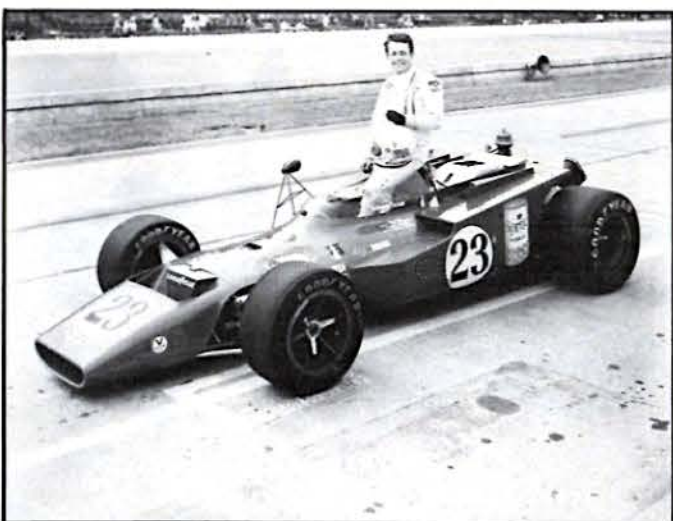
Car No.: 23 Driver: Mel Kenyon (Sprite Spl.) Qual. Speed: 170.205 Day: 4 Start: 30th Finish: 32nd Entrant: Lindsey Hopkins Chief Mechanic: Don Kenyon Engine: Ford Turbo Plugs: Champion Tires: Goodyear Front size: 10.40 x 15 Rear size: 15.70 x 15 Chassis: Kuzma-Kenyon Engineering features: Re-located oil tank-wedge type design Driver's previous finishes: 5th '66; 16th '67; 3rd '68; 4th '69; 16th '70* History of car (Year, driver, qual.speed, start, finish, etc.): New Car Money won: $14,153 Laps completed: 10 (wrecked in Krisiloff crash) *Relieved by Roger McCluskey
