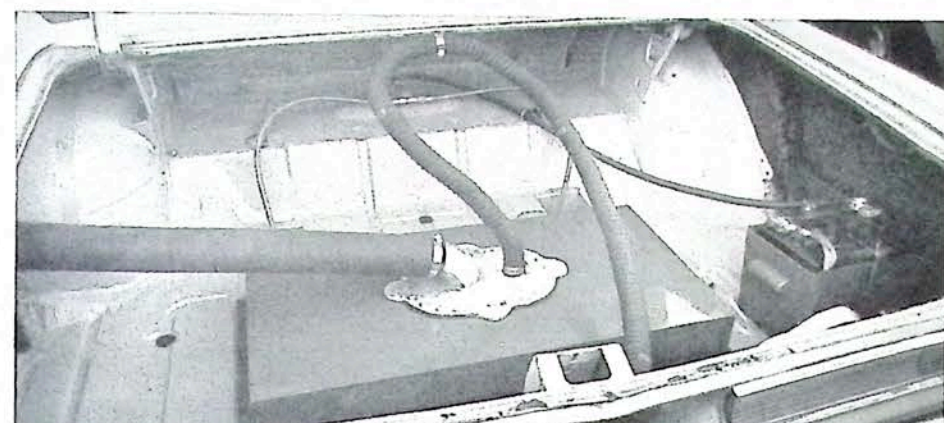
Above: Fuel system uses 22-gallon Firestone fuel cell and two Holley centrifugal fuel pumps. Two batteries are now carried to aid traction out of turns. Below: Interior is less sparkling, but driver Bob Tullius finds it livable. Collapsible steering column and tilt wheel are out of late GTO. Homemade bucket seat gives lateral support needed for the Tempest's 1.1g cornering.
