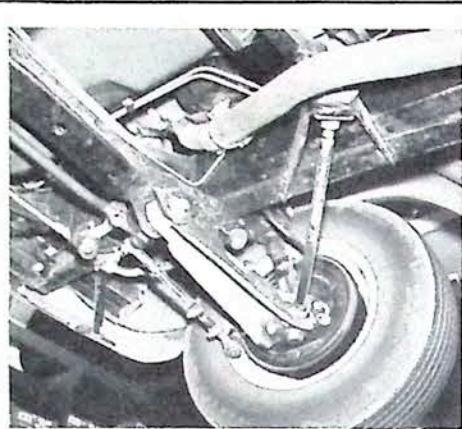
IH has modern strut suspension, torsion bars. Or, if you prefer, opt for parallel leaf springs.
