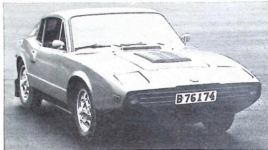
Saab Sonnet is front-wheel-drive sports car intended mainly for export. Engine is 1500cc V4.
