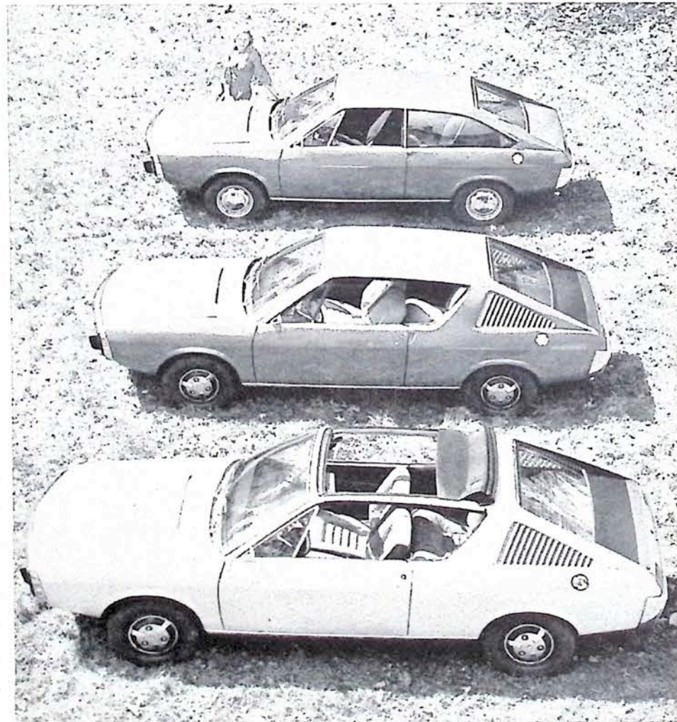
Three variations on Renault's sporting theme, the top being your basic small-engine 15 coach. In the middle is the 17 coupe and at the bottom, the 17 "decouvrable." Body variations are matched by list of engine, brake, transmission, interior options. Car uses Renault 12 chassis.
