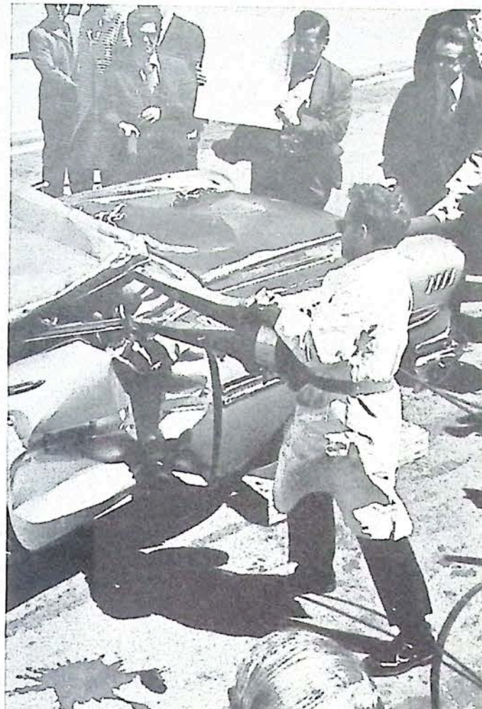
Still in the prototype stage, the Hurst tool can easily be handled by one man and is compact enough to fit in the equipment lockers of most modern rescue vehicles. If retailed, it will be sold for $3-400.
