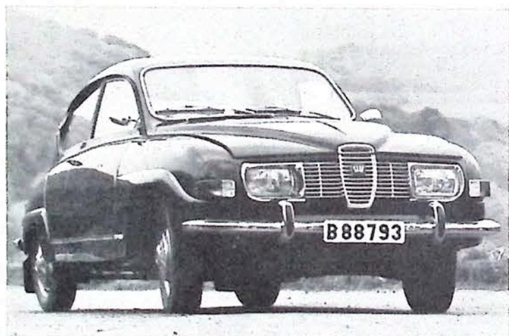
Saab 96 is latest version of company's first offering back in 1947. Unit steel body, front-wheel-drive, smooth shape are still trademarks.
