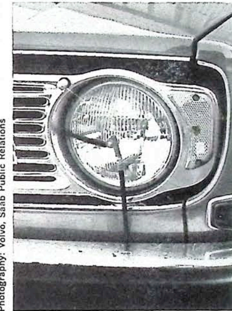
Above: Saab's headlight wiper/washer combination incorporates miniblade and horizontal action. Above right: Volvo goes a different way with circular blade sweep U.S. may see these by '72.
