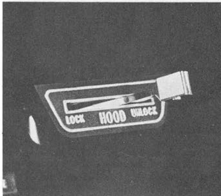
ABOVE—The under dash hood lock unit will keep prowlers out of the W-30 motor.
