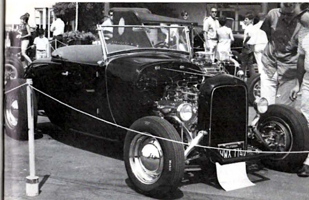
Dick Megugorac of Magoo's Auto Shop built this '29 highboy using Chevy power, a '39 trans and rebuilt '32 rear end. He drove it thousands of miles with no problems, and present owner reports complete reliability.
