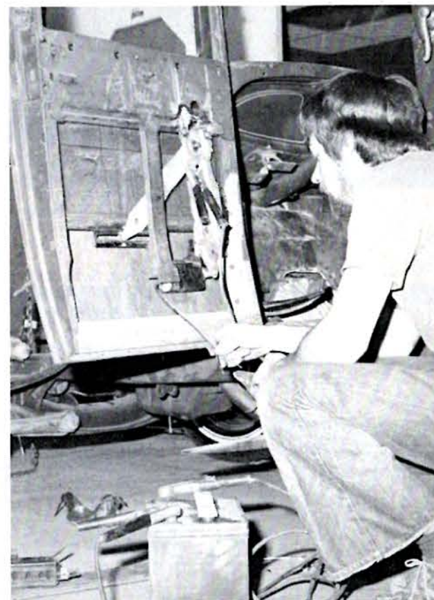
Before going any further, Ron yanked out a battery and jumper cables to test his handiwork. Presto! Power windows without a hitch.
