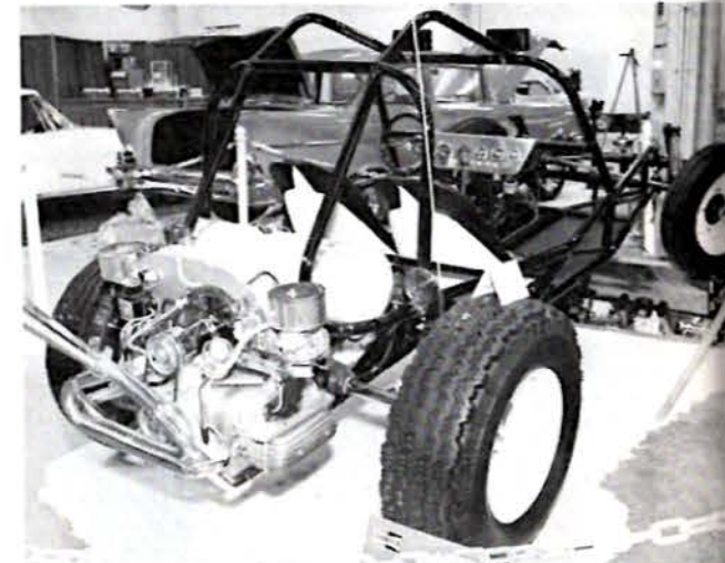
This Sand Buggy built up by Luther Graham from Louisville, Ky., runs about with rear-mounted 1800cc VW four-banger. Space chassis features coils and torsion bars up front.
