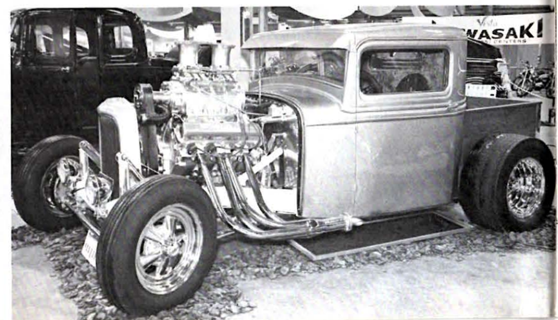
Mike Brooks of Fairdale, Ky., is the builder of this '32 Ford pickup mounting a 455 Olds powerplant. Blower used is popular 6-71 model, tranny is T-10 mounted with Chevy rear axle and 4.11 rear gear.
