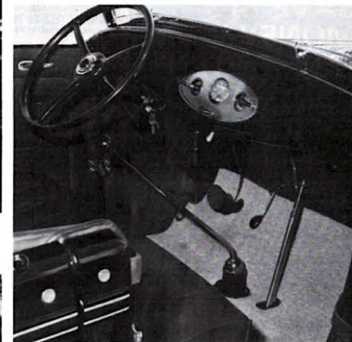
Inside and out, the car retains its stock appearance. Transmission is a '39 Ford unit. New carpet covers natural-finish wood floorboards.
