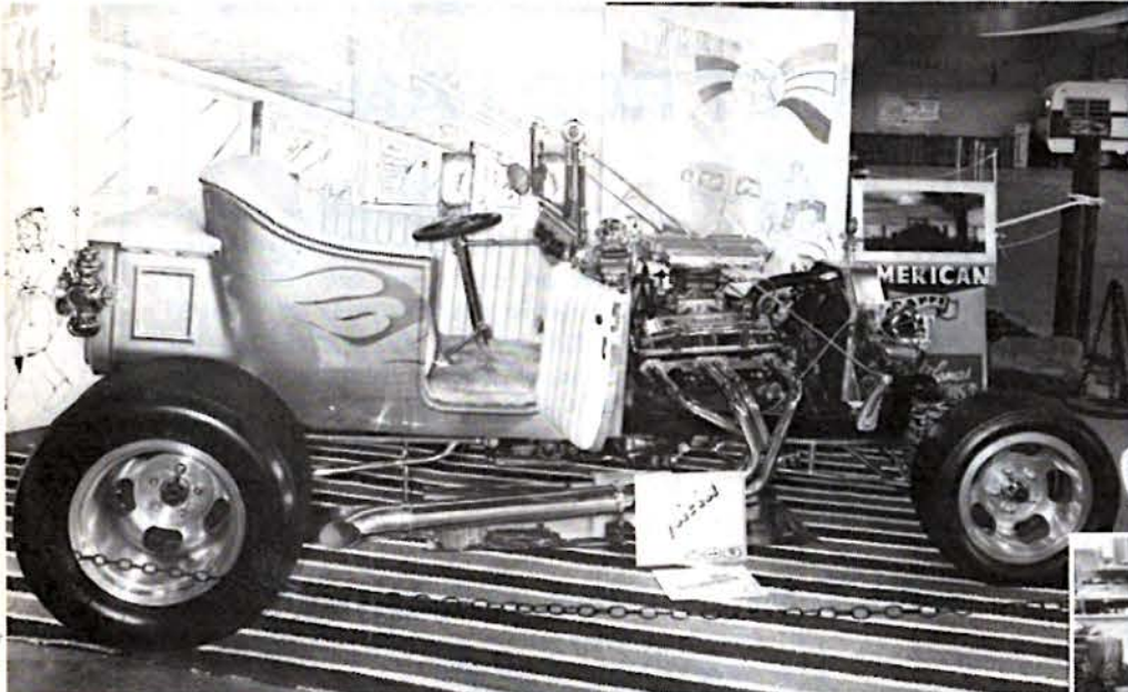
Nifty 1915 Ford T is owned by Bill Thomas of Evansville, Ind. Coil suspension on a tube axle is featured up front. Car also has brass radiator, chrome running gear, handmade radius rods and coils on the rear axle.
