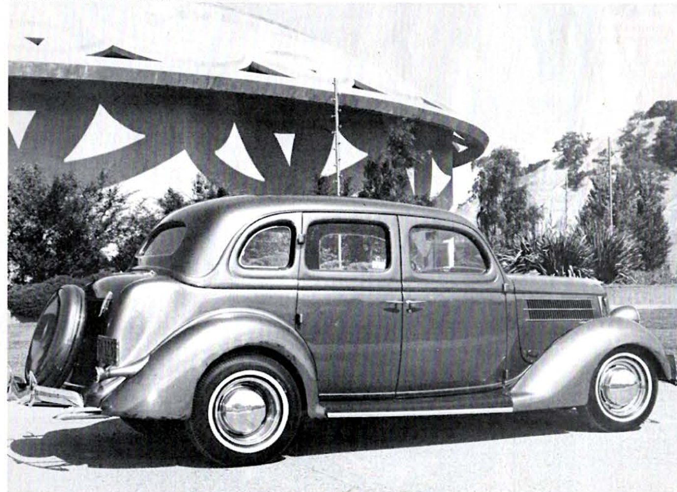
Front axle has been dropped 3½ inches so car sits on rake. Those are chrome '50 Merc steel wheels (reversed in the rear). They're shod with Firestone tires.
