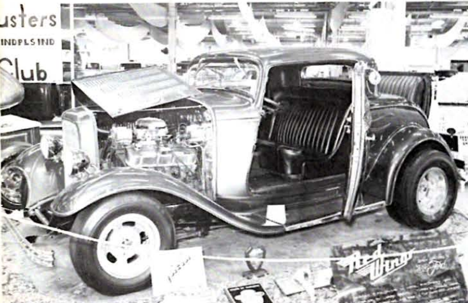
Pretty '32 Ford coupe shows off a four-inch top chop, 402 Chevy engine with a 400 turbo, 4.10 rear axle. There are 290 louvers in that hood! Owner is Don McNeil from Indianapolis, Ind.
