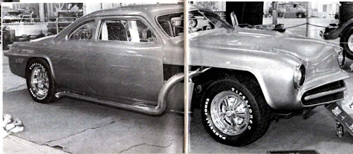
Haven't seen one of these for some time: a 1950 Ford. This one, the "Bushwacker," was built up by Ron Linder, Louisville, Ky. The engine is a 390 Ford. Car has been sectioned six inches and chopped four-and-a-half. Frame has been chopped front and rear a total of six inches. Wheelwells have been reworked, rear section frenched, front end has rolled metal tube construction. Dash panel is sectioned '56 Ford item.
