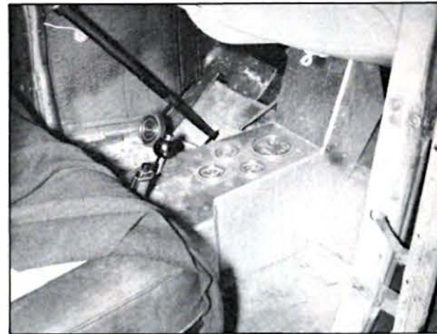
This Model A is powered by a V-8 and automatic—which meant surgery in the floor area. This all gets hidden by a very functional console, shown here partially finished. A solid idea for many an early rod.
