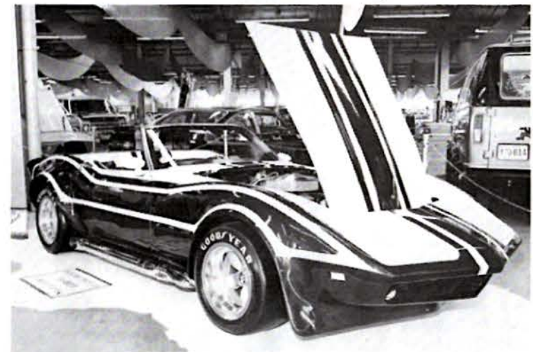
This 'Vette is owned by Larry Bobziem from Louisville, Ky. Side pipes have been added as well as reworking of the front and rear sections. Engine is a 327-incher.
