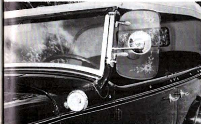
Etched glass windwings are the work of Richard Dannebaum of Classic Glass in Whittier, Calif. Top needed all new wood for bows.
