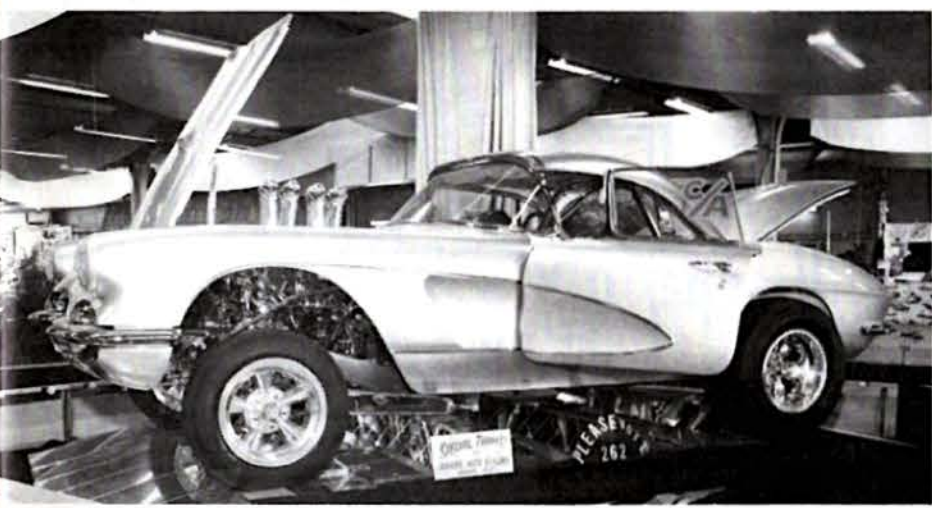
One of the big winners of the show was this 1961 Corvette built up by owner Wayne Gelfman from Charlotte, Pa. Interior has crushed velvet stitching, roll bar. Front end features tube type axle and chromed chassis and engine parts. Green pearl paint highlights this comp classic.
