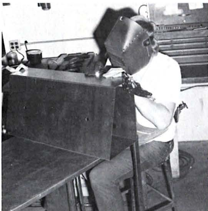
If you can't hell-arc, then short arc will work. This wire feed method is commonly used in header shops.
