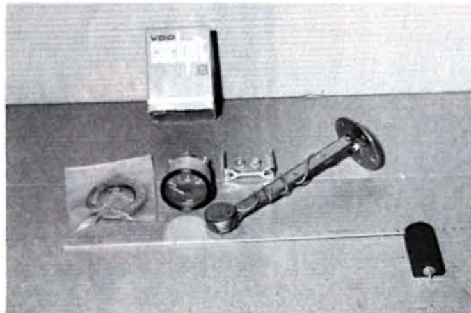
Instrumentation for the Project Roadster was handled with VDO gauges. The Cockpit series was selected. Here the fuel gauge with all the necessary hardware, float, pickup and instructions is ready. It is an electric gauge with light.
