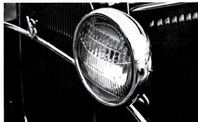
All that is left is to replace the rim and lens assembly. Be sure to hook the rim over the tabs and secure the catch.
