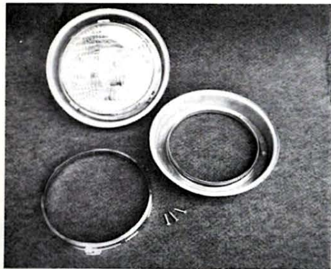
The sealed beam conversion kit consists of two spacer rings and two clamping rings and the screws to hold them together. The first step is to install a sealed beam (not included) into each ring set.
