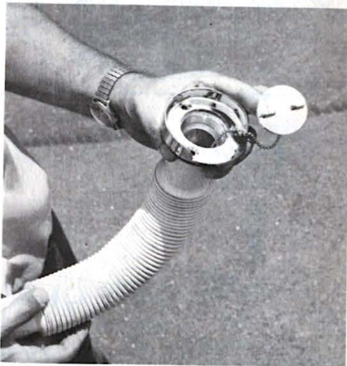
Demonstrated is the TP gas filler assembly, note the safety chain. Filler is flush mounted and held in position with three counter sunk screws or bolts. Cap also fits flush.
