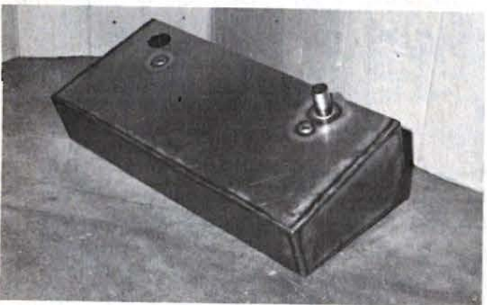
The finished product. The custom gas tank holds 15 gallons and was made from 16 gauge mild steel and weighs approximately 135 pounds when full of fuel.
