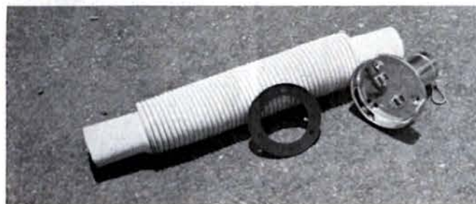
Additional accessories needed to complete the gas tank are hose (neophrene type), gasket and filler neck with cap. All this comes in a kit from Total Performance. The hose is gas resistant and the cap screws on with a safety chain for added protection.
