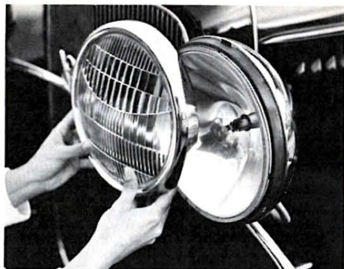
The headlight rim and lens is removed, and then the reflector assembly. A new wiring harness must be installed so that the sealed beam can be plugged in.
