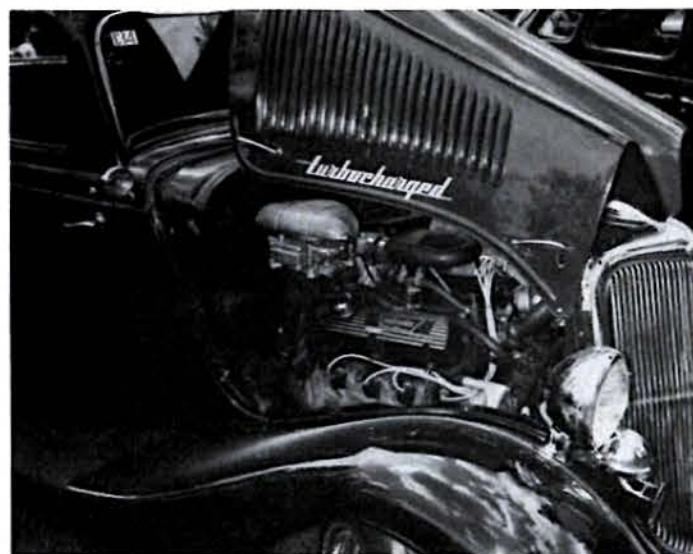
Unusual turbocharged engine in 1934 Ford coupe was quiet and dependable. Turbo blowers have yet to make it big with street rodders, but they work well.
