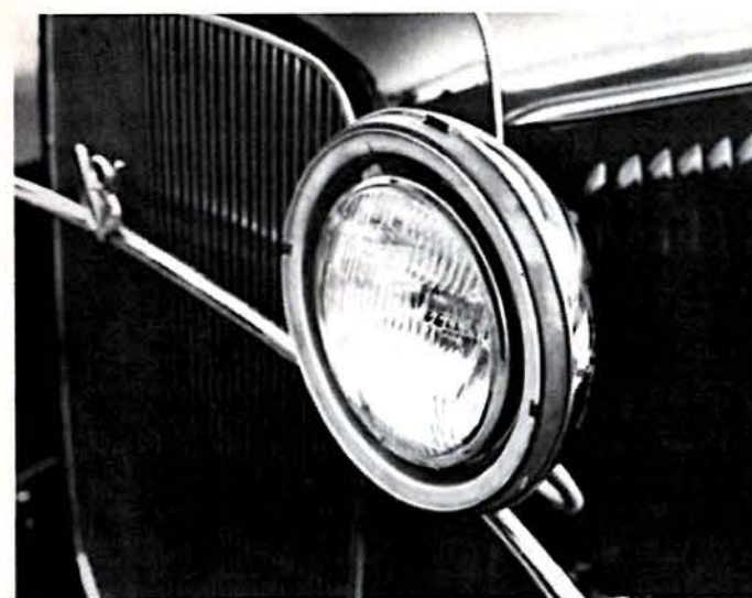
The new assembly is now installed and the wiring connected. Note that the spacer centers the sealed beam in the headlight bucket.
