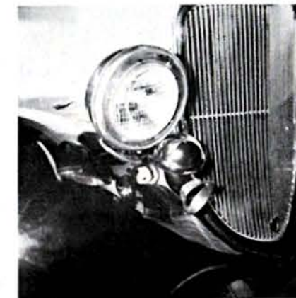
At one time, this was the type of sealed beam conversion kit available. It works fine, but it is not nearly as appealing. To some it is downright ugly.
