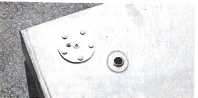
VDO sending unit can be installed with the tank all welded and in a completed state. Unit is well made and easy to work with.
