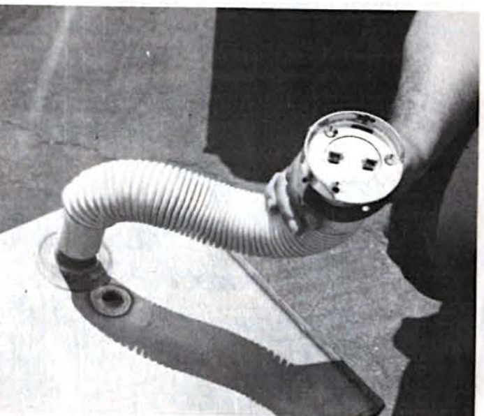
Hose has 1 1/2-inch opening on either side, make sure to note this when making gas tank and use proper inlet size tubing. Eighteen gauge mild steel tubing does the job.
