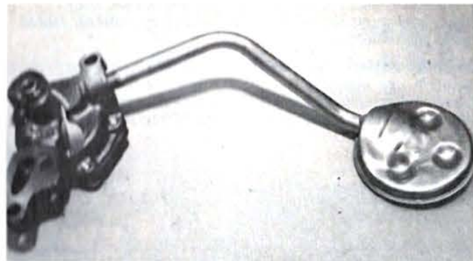
Mopar "A" engines need help in the oiling department. Large diameter pump pickup tube and high volume pump must be installed.
