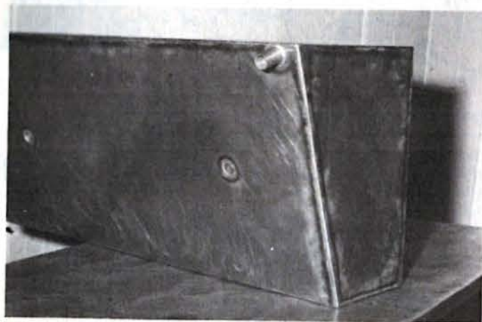
Outlet was made from a piece of 3/8-inch pipe. Depending on engine size a 1/4-inch pipe fitting could also have been used.
