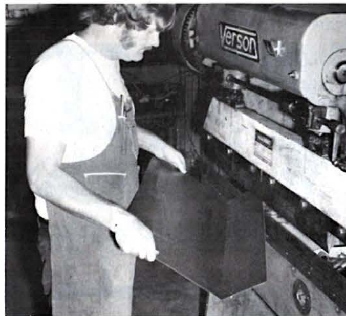
Unless you're very lucky you won't have one of these nifty sheet metal benders, so you have two choices. First check out your local air conditioning shop, if any, as they should have this type of bender or use angle iron, heavy steel or channel and place the gas tank material between it. Make sure to C-clamp the ends to prevent movement and use a soft mallet to bend the material.
