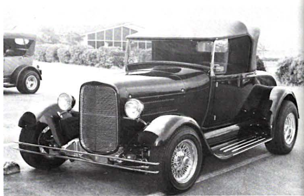
Gil Ferriera's '29 Model A was one of the meet's finest. Horizontal bar grille in '32 shell, aluminum hood, running boards, trick headlight bar, and twin-bar bumper were several of many construction details.
