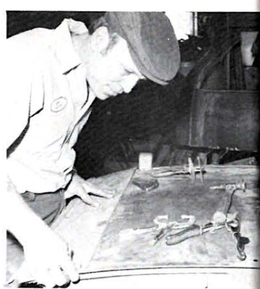
Expert bodyman Bob Barr lends a hand in the fitting of new sheet metal panel to lower portion of T's door.
