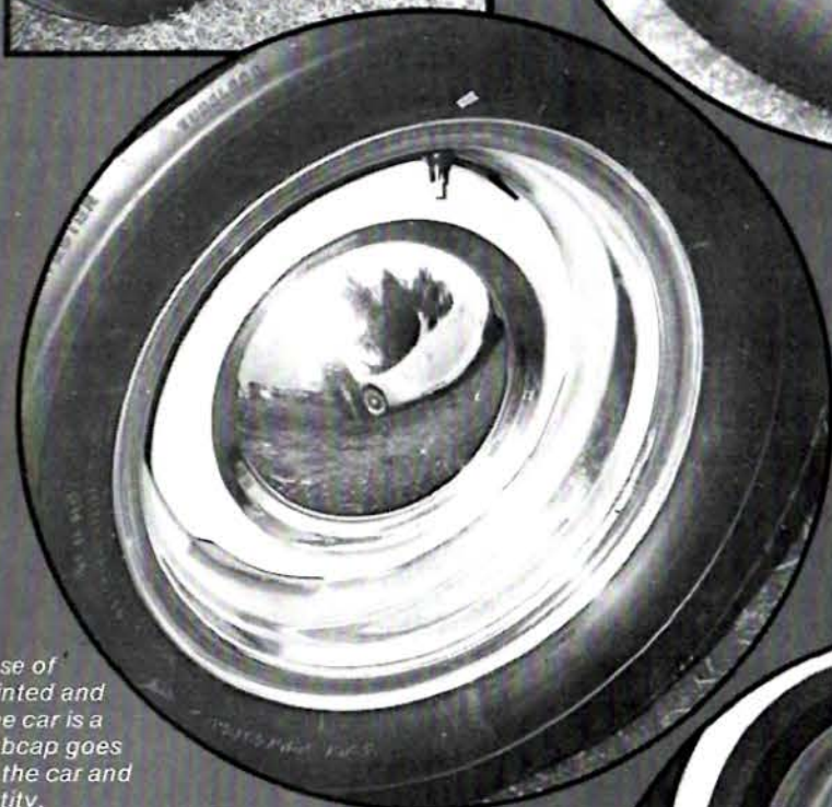
One more variation of the Chevy rallye wheel. This one features a larger baldy type cap and instead of paint, center has been anodized to contrast with body color.
