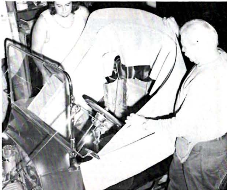
After the back panel is finished, it's glued to wood insert and the top edge is stapled firmly to the insert to make sure it's held tightly all along the top because this finishes off the top of the diamonds.
