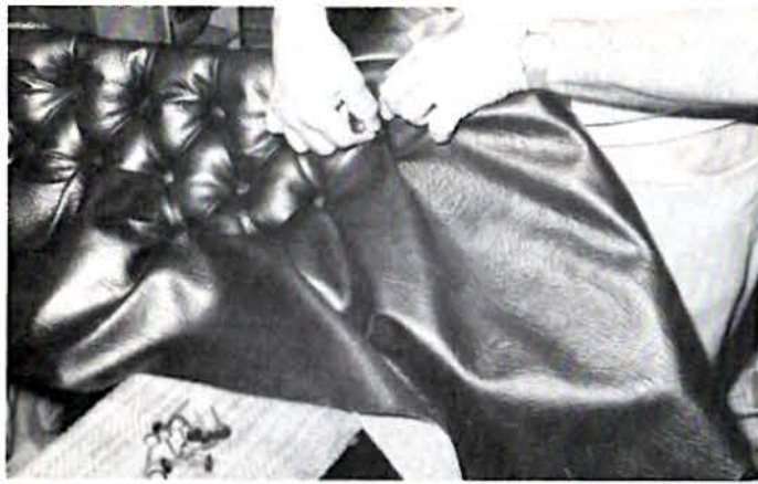
After the Dacron filler is in place, a #22 prong type button is shoved through the material and a hole in the foam with the prongs bent over the backing. This is done for each diamond pleat.
