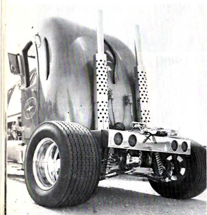
Cecil the Diesel, a hand-built mini-truck that tows a show rod on a flat-bed trailer, is powered by a Mercedes-Benz four-cylinder diesel engine. Chrome Jaguar rear end, big stacks, jaunty cab, side gas tanks, and of course a CB radio, add to truckin' flavor.
