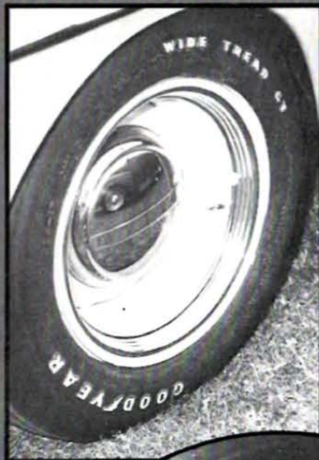
Here's the painted Ford wheel one more time. This one has been reversed for wider base but still retains small Ford cap and beauty rim combination.
