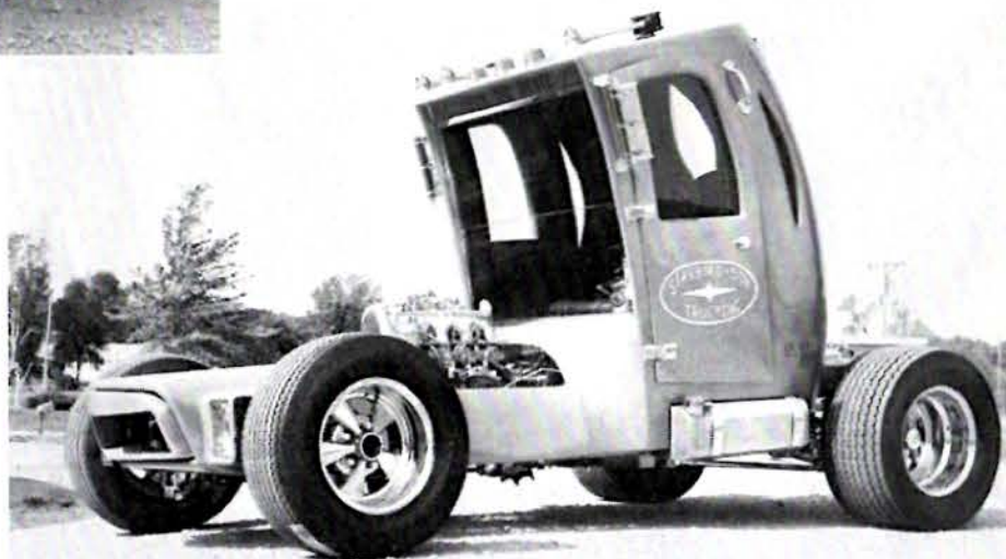
Cecil the Diesel, a hand-built mini-truck that tows a show rod on a flat-bed trailer, is powered by a Mercedes-Benz four-cylinder diesel engine. Chrome Jaguar rear end, big stacks, jaunty cab, side gas tanks, and of course a CB radio, add to truckin' flavor.
