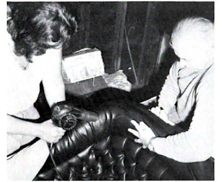
Start at the corners when pulling up the covering material for the roll. This area is the hardest to fit. Work out the folds with a hair dryer gun to heat up the material and make it pliable.
