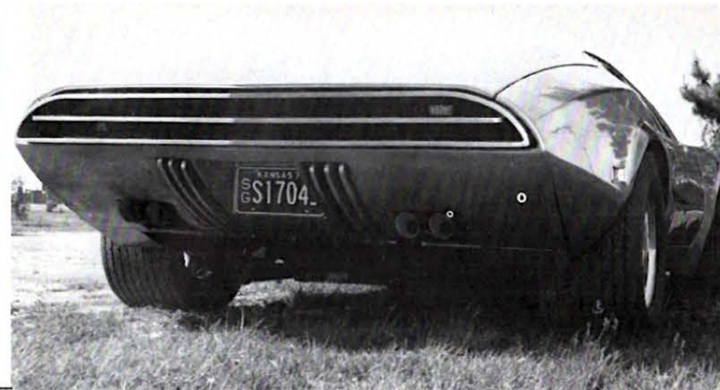
Latest Starbird creation is a wild Panthera with much hand-formed sheet metal. Rear quarter panels have been widened five inches to accommodate wide rubber and reshape the quarter windows. Nose is extended a foot with a full-width aluminum grille and front fenders are also widened. Pearlescent gold, scalloped coupe is powered by a 6:71-blown, Enderle-injected 351 Ford engine.
