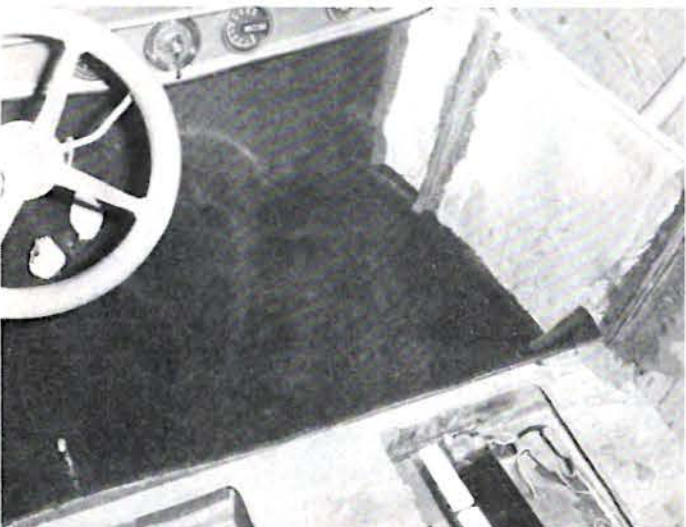
Carpet should be installed before the insert is placed into the body. Edges of the carpet are hidden which gives a better finished appearance.
