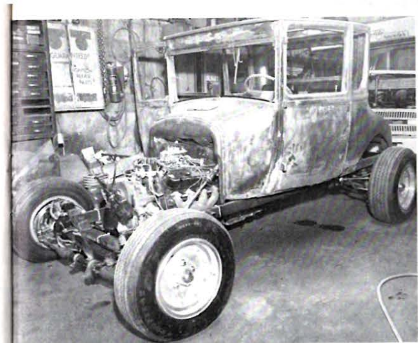
The custom-built frame required little modification to mate it to body. The firewall has been recessed so original full hood will fit over 302-inch '74 Ford small-block. Engine has been set back a total of 10 inches, also improving weight distribution.
