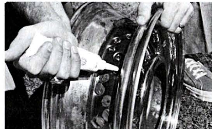
After the primer has dried for a minimum of one hour at approximately 70°F., carefully work Silicone rubber (RTV) into the nipple area around each spoke. Make sure to eliminate any bubbles or air pockets.
