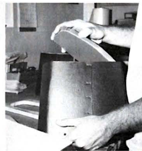
The end piece for the liner is die cut also, and is then formed in a press to give smooth folds. Fit must be exact to give a finished look.
