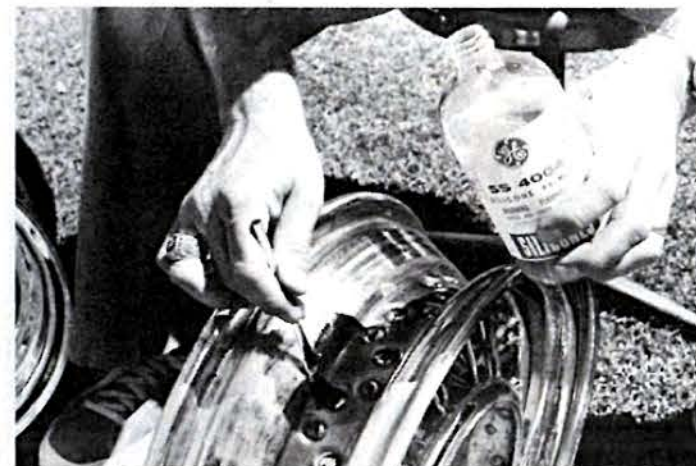
After the wheel is perfectly dry, the GE SS 4004 silicone primer is applied using an acid brush. An even coat is required as this is what prepares the non-silicone rubber surfaces for the RTV to be applied.
