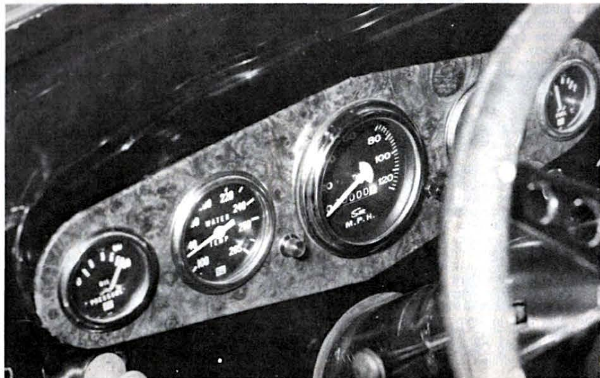
A new speedometer is only half of what is needed to get the numbers on your speed and miles traveled, a drive unit on the transmission is also needed.
