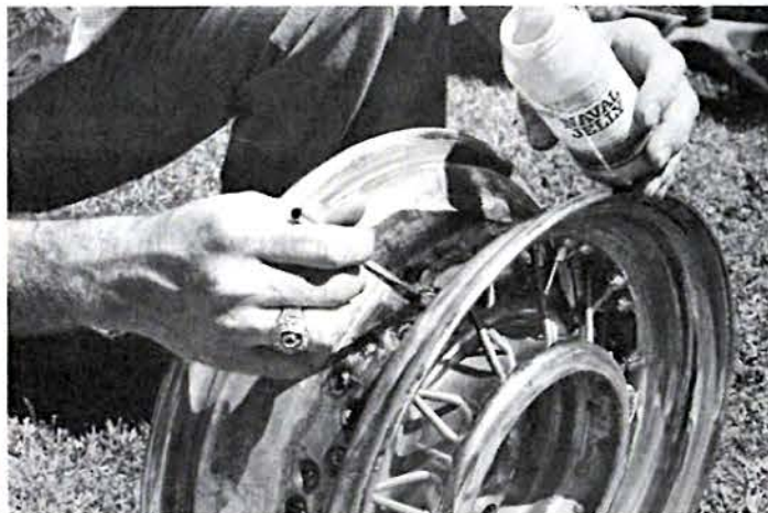
There is usually a layer of rust around the nipples, due to the band holding moisture in. Here we used an acid brush to put on the Naval Jelly, this area must be cleaned completely.
