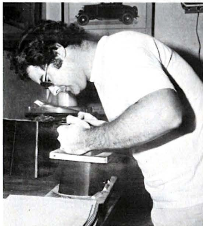
A clamping form is slid over the formed liner to keep it in place for the stapling step.
