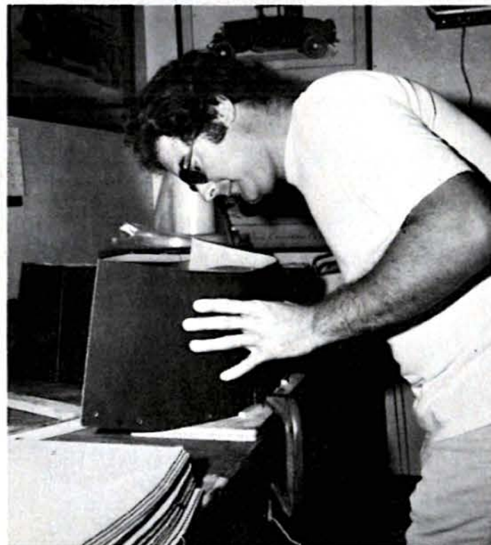
Each die cut glove box liner is formed around a special wooden block. Exact shape is assured on each unit.
