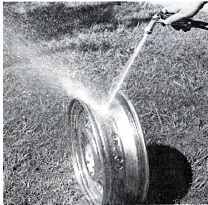
Plenty of water under high pressure is needed to remove the rust and Naval Jelly. Steps 2, 3, and 4 may have to be repeated if the rust is very bad.
