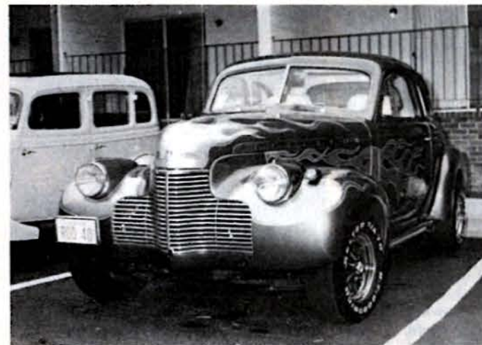
Bill Tilley of Richmond, Virginia, drove his 1940 Chevy coupe, sports flames, powered with Chevy 327, turbo 350.
