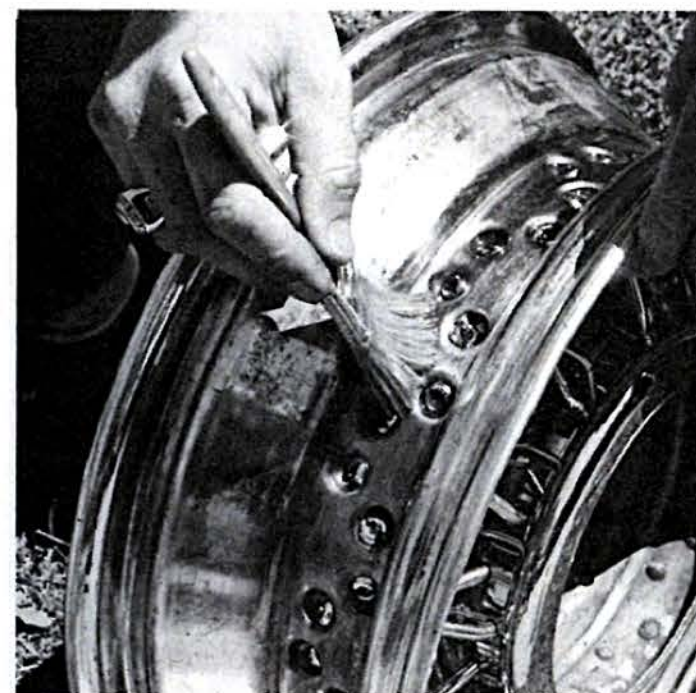
A regular 1 1/2 inch paint brush works well for applying the solvent. Keep in mind that the quality of the finished product depends on how clean the area around each nipple is.
