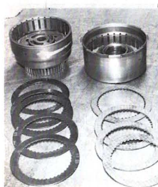
11. These two types of clutch plates must be installed in their respective clutch cylinders, easily identified by a smooth or a waffle lining.
