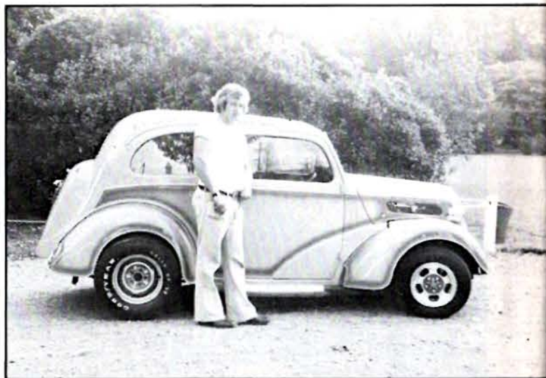
Paul Williamson's yellow and red Ford Pop has a flip frontend hiding a 302 Ford mill which drives through a narrowed Mustang rear.
