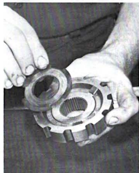
3. A thrust-washer gets placed between the case and the parking pawl gear. Use a little (white) grease whenever the washers need to be held in place.
