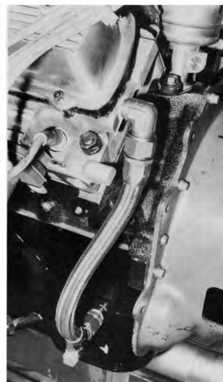
Olds/Batten competition heads have 1/2-inch provisions at each end to accept drainback plumbing.
