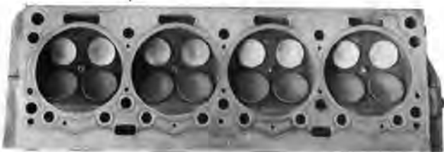
Cut-away cylinder head section illustrates the shallow valve angle and the extensive coolant jackets surrounding the valves. Unique chamber design called for a maximum ignition timing of 29-30 degrees, while production Rockets called for a more conventional 37-38 degrees of spark lead.
