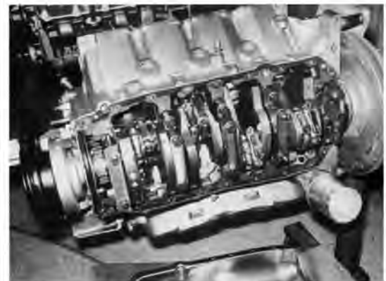
The special iron and aluminum cylinder blocks cast for these experimental engines were the first factory Rockets fitted with four-bolt main bearing caps. Produced entirely in iron, the pushrod W-43 engine weighed 86 pounds more than a stock 455. With an aluminum block and cylinder heads, the same assembly weighed 75 pounds less than a stock 455. Produced solely as an all-alloy combination, the OW-43 cammer weighed 50 pounds less than the same stock 455.
