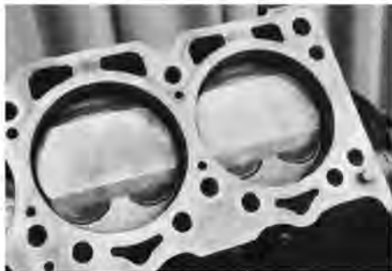
Although both cast and forged pistons were made for these engines, dynamometer evaluations were conducted using these 10.2:1 forged-aluminum units. Designed to allow maximum practical squeeze with minimal flame-front obstruction, these forged-alloy slugs incorporated carefully contoured tops.
