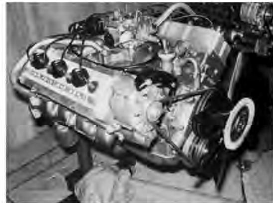
Designated W-43, this engine's mile-wide valve covers hint at the Chrysler-style science that resides within. Cast in iron, like its 455-cubic-inch production counterparts, this prototype Rocket spewed out 550 hp at 6500 rpm with the help of hemispherical combustion chambers, four valves per cylinder, a high-capacity four-throat Quadrajet carb, special-cast crankshaft, forged-steel connecting rods and 10.2:1 high-squeeze pistons. According to Oldsmobile engineering sources, the W-43 engine was the one powerplant in this experimental series that came closest to actual production.
