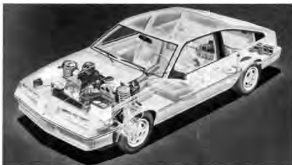
This phantom view of a late-model Firenza illustrates the transversely mounted front-wheel drive engine/trans module and the widely spaced MacPherson struts. Efficient packaging provides handling, performance and plenty of room inside.
