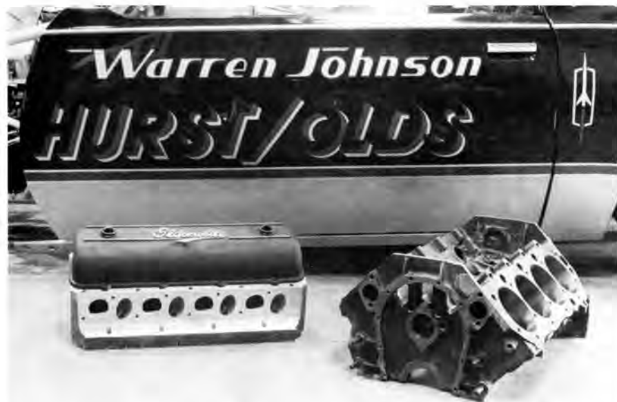
Oldsmobile's current competition efforts are centered around two basic castings: a highly refined iron-cylinder block (part No. 22521056) and a state-of-the-art, high-tech aluminum cylinder head (part No. 22522055). The pieces shown here propelled Warren Johnson's 1983 Hurst/Olds into the NHRA World Finals winner's circle. A second batch of head castings introduced early this year featured revised port and runner arrangements, reduced weight, better metallurgy and other structural improvements.
