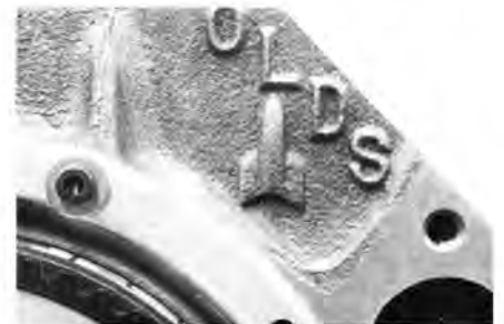
Visibly similar to an earlier GM iron V8 casting, a close inspection of this latest Oldsmobile Rocket will reveal the beefier features that help make it a nearly bulletproof race motor. The deck surfaces are nearly an inch thick and the bores are siamesed for superior structural strength. Eight additional cylinder head clamping bosses have been cast into the valley just below the deck surfaces. Along with the eight corresponding bolt holes located along the lower edge of the deck face, they form a solidly sealing, evenly spaced six-bolt clamping pattern around each cylinder. Production blocks are now also cast in aluminum, and all have the Olds Rocket emblem cast right into the block.
