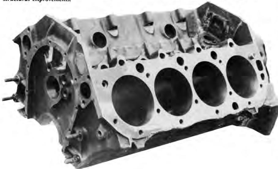
Oldsmobile's current competition efforts are centered around two basic castings: a highly refined iron-cylinder block (part No. 22521056) and a state-of-the-art, high-tech aluminum cylinder head (part No. 22522055). The pieces shown here propelled Warren Johnson's 1983 Hurst/Olds into the NHRA World Finals winner's circle. A second batch of head castings introduced early this year featured revised port and runner arrangements, reduced weight, better metallurgy and other structural improvements.
