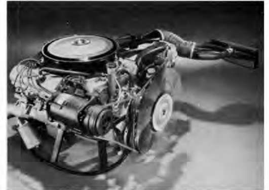
Production excitement took many forms. Hot Toronados rocketed up Pike's Peak and smoked all four tires on the dragstrip. Underhood, the Toro model was far from ignored. This 1968 force-air production option included longer cam timing, heat-treated valve springs and hot rod-type distributor modifications to pull 400 horsepower from the Toronado's 455 V8.
