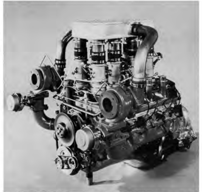
Far from its original production form, this Olds 455 led the Rocket's attack on the Can-Am series. Some of these lightweights were overbored to 503 cubic inches! This all-aluminum 455 used Lucas fuel-injection and twin TRW turbochargers to make 659 horsepower and 554 foot-pounds of torque.
