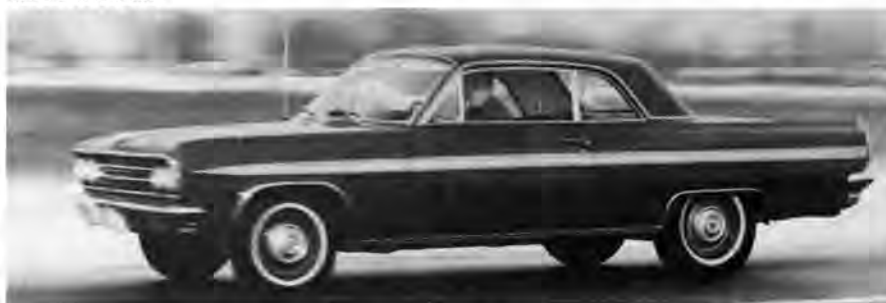
When Olds elected, in 1962, to turn its totally tame F-85 V8 intermediate coupe into an on-demand tarmac terror, the Jetfire was the result. With the addition of a Garrett-AiResearch turbocharger to the division's 215-cubic-inch lightweight aluminum V8, the resulting Turbo-Rocket motor cranked out one-horsepower-per-cubic-inch!
