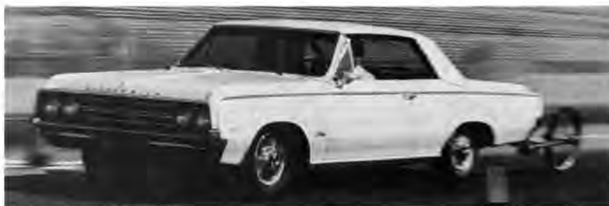
Available in any F-85/Cutlass model (except a station wagon), a total of only 2999 4-4-2 options rolled out of the factory in 1964. The 4-4-2 designation indicated a four-barrel carb, a four-speed trans and rumbling dual exhausts. Fitted with already-available extra-duty hardware that included enforcement-oriented springs and shocks, a new rear stabilizer bar, a dual-snorkel air cleaner and low-profile 7.50x14 red-stripe sidewall tires, the first 4-4-2 option was actually listed as a "B09 Police Apprehender Pursuit" package.
