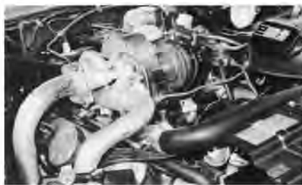
When Olds elected, in 1962, to turn its totally tame F-85 V8 intermediate coupe into an on-demand tarmac terror, the Jetfire was the result. With the addition of a Garrett-AiResearch turbocharger to the division's 215-cubic-inch lightweight aluminum V8, the resulting Turbo-Rocket motor cranked out one-horsepower-per-cubic-inch!
