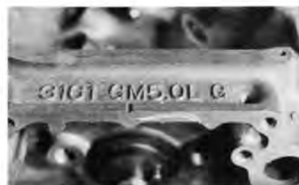
For identification purposes, 1977 and later castings and all of the lightweight 350s have their displacement cast into the side of the cylinder block. Other late V8s indicate the year they were cast by a numerical designation forward of the intake manifold rail (arrow). A single letter cast there indicates a big-block, while a single digit stands for small-block. Numbers 3 through 7 indicate the really good small-blocks. A single letter followed by a single digit number designates a 403. The 5L and 5.0LG both indicate a 307-inch gasoline block. The 350DX marking designates a 350-cubic-inch diesel block while the 403 speaks for itself. Olds service manuals also offer clues to the casting codes.
