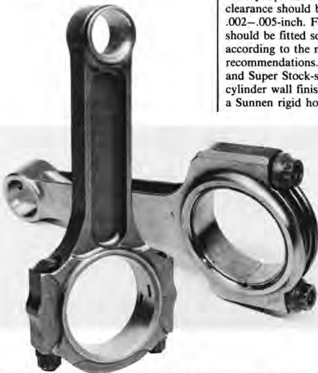
When the rules allow them and where the power demands them, aftermarket steel connecting rods from Crower or Carillo and high-strength big-end hardware by SPS can help make an Olds reciprocating assembly practically bulletproof.
