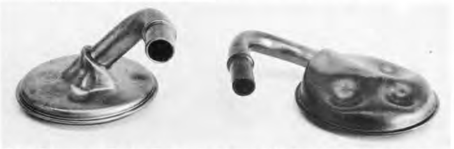
High-performance modified small-blocks can also use a 427 Chevrolet passenger car oil pump pick-up pipe and screen assembly (left). It has a larger ( \frac{7}{16} -inch) inside diameter (as opposed to the standard Olds \frac{1}{4} -inch) for increased lube moving capacity. An engine fitted with a larger "sucker pipe" will benefit from increased volume rather than increased pressure.
