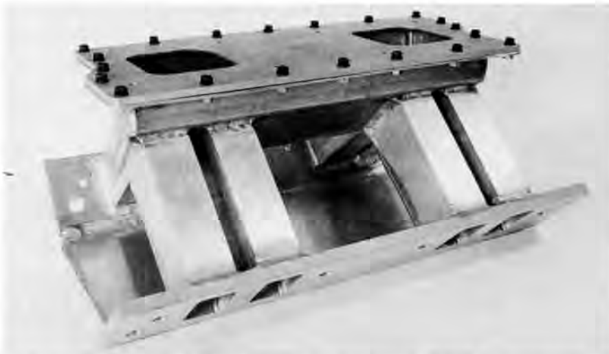
Olds enthusiasts interested in all-out performance can now avoid the $1000-plus price tags of custom-fabricated manifolding. This aluminum tunnel ram manifold from Precision Speed has a removable top to accept a pair of standard Holleys, twin 4500 Dominators or a single 4500 Dominator carb. They're made to fit 350- or 455-cubic-inch engines with either stock or Batten cylinder heads, without requiring spacers or adapter plates.
