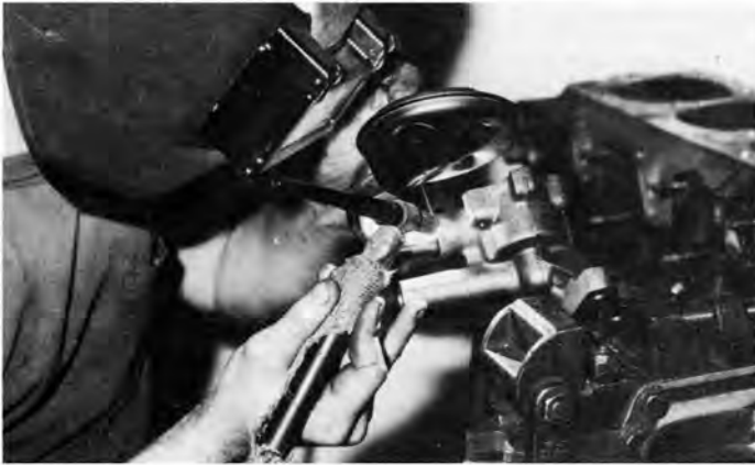
The Toronado pump inlet must be enlarged from \frac{1}{16} -inch to \frac{1}{8} -inch to accept the fatter Chevy tube, which is then repositioned 180 degrees, pressed into the Olds pump body and welded in place. For reference, the Toronado pump is rated at 25 gpm, free volume.
