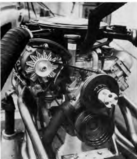
Production W-31 350 engines used in 1968-'69 were select-fit assembled and dyno-tested before installation. Factory-rated at 325 hp at 5600 rpm, each one of these W-series small-blocks was actually evaluated in the Olds engine labs to be sure it delivered. Notice how the dyno motors were fully dressed (with all pumps, alternator and air cleaner) while tested.
