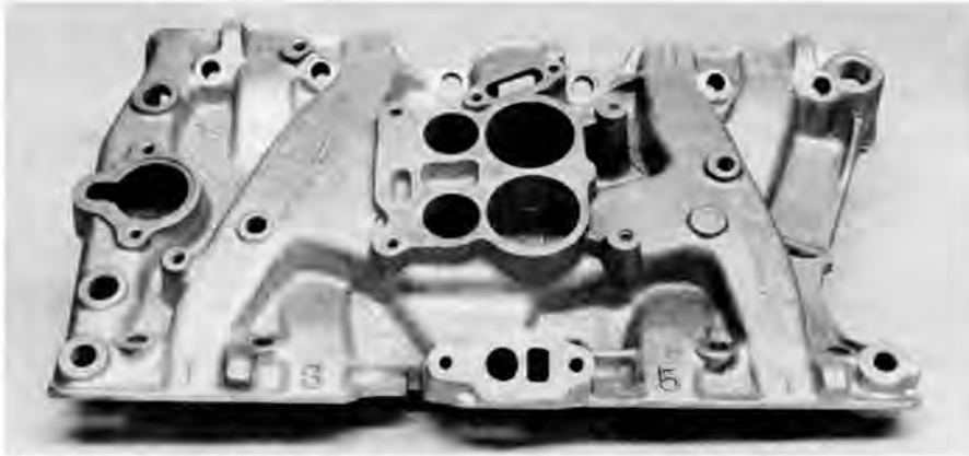
Most late lightweight V8s fitted at the factory with a four-barrel carb use this low-profile, dual-plane alloy casting. Earlier high-rise versions of this 180-degree manifold, as well as most of those produced by the aftermarket, are more capable performers. This unit was designed to produce low-speed response and fit beneath a low hoodline.
