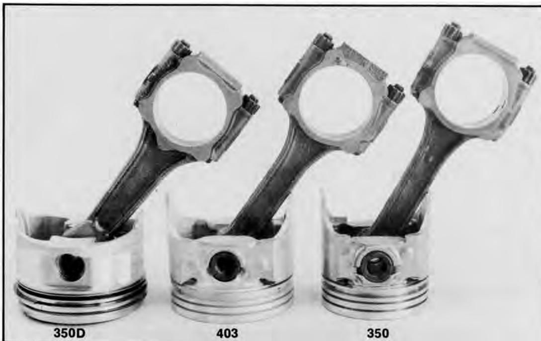
Although the 403 connecting rod (right) is considerably larger across its beam section, it can be trimmed to a 350 rod's weight by careful machining of the balance pad at its big end. A Tufftriding treatment can help make any Olds rod more durable in an extra-duty application. Note the large oil depressions in the pistons below the bottom ring lands (arrows) which leave the skirts relatively unsupported.
