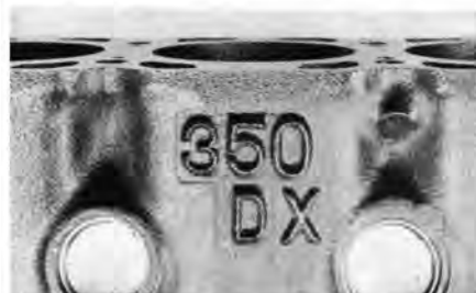
For identification purposes, 1977 and later castings and all of the lightweight 350s have their displacement cast into the side of the cylinder block. Other late V8s indicate the year they were cast by a numerical designation forward of the intake manifold rail (arrow). A single letter cast there indicates a big-block, while a single digit stands for small-block. Numbers 3 through 7 indicate the really good small-blocks. A single letter followed by a single digit number designates a 403. The 5L and 5.0LG both indicate a 307-inch gasoline block. The 350DX marking designates a 350-cubic-inch diesel block while the 403 speaks for itself. Olds service manuals also offer clues to the casting codes.
