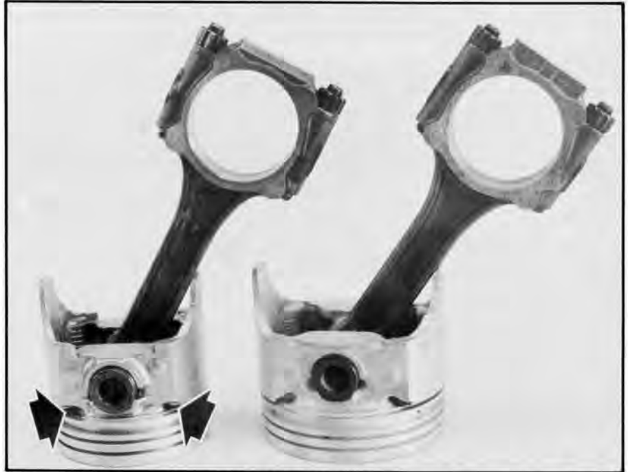
Although the 403 connecting rod (right) is considerably larger across its beam section, it can be trimmed to a 350 rod's weight by careful machining of the balance pad at its big end. A Tufftriding treatment can help make any Olds rod more durable in an extra-duty application. Note the large oil depressions in the pistons below the bottom ring lands (arrows) which leave the skirts relatively unsupported.
