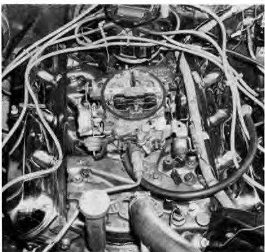
Retaining most of its external OE equipment, including the stock airflow-limited Quadrajel carb in this late-Seventies/early-Eighties A-body Olds, the 350 small-block is a more-than-capable 12-second quarter-mile performer. The next logical step up for this modified small-block Rocket involves breathing tweaks based on aftermarket intake system parts and refined original equipment.
