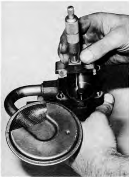
High-performance modified small-blocks can also use a 427 Chevrolet passenger car oil pump pick-up pipe and screen assembly (left). It has a larger ( \frac{7}{16} -inch) inside diameter (as opposed to the standard Olds \frac{1}{4} -inch) for increased lube moving capacity. An engine fitted with a larger "sucker pipe" will benefit from increased volume rather than increased pressure.
