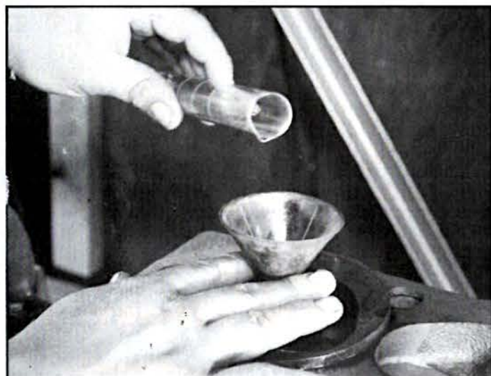
Combustion chamber volume checked out at 117 cc's. This yields a streetable 8.2 to 1 compression ratio when used with TRW flat-top pistons and Mr. Gasket composition-type head gaskets.
