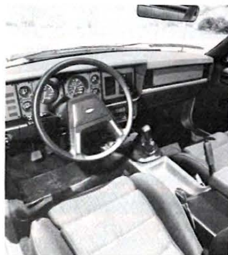
The '84 GT 350 interior is much the same as a stock Mustang GT. Real gauges (a luxury these days) grace the dash, along with an analog speedometer and tach.
