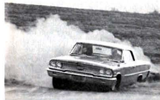
Offered with the optional early-model 406- and, later, 427-inch big-blocks, it's no wonder Ford's best seller in '63 was the Galaxie. Despite their excessive weight, the Galaxies still held their own on the street.
