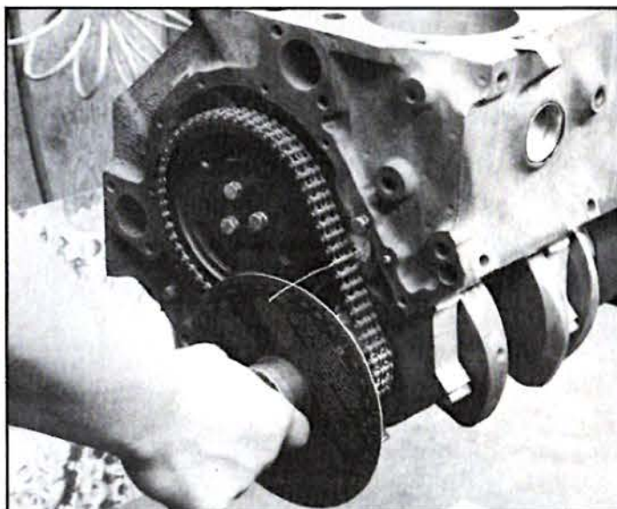
After finding TDC of the number one piston, we were ready to degree our cam. Our Isky piece features 286 degrees duration, .510-inch lift, and 108-degree lobe centers, and was installed straight up using a Cloyes three-position true roller timing chain set.
