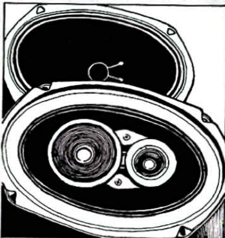
Replacing inferior stock 6 x 9 speakers (top) with aftermarket three-way speakers (bottom) results in an instant improvement in sound quality for a relatively low price.
