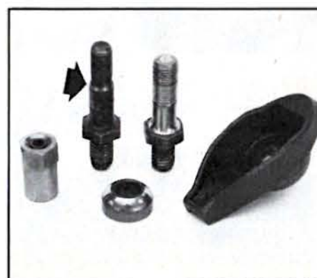
Desirable early-model cylinder heads have threaded bosses for rocker arm studs (left); later castings have notched pedestals (right). These heads can be converted by milling the pedestals, then drilling and tapping the holes for studs.
