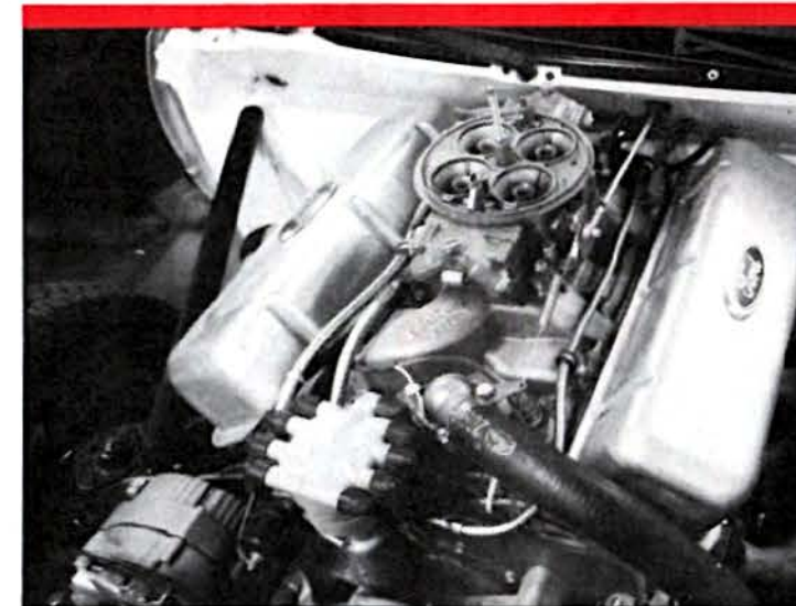
With a blue oval displayed prominently on the valve covers and a front-mounted distributor, most folks would think that this is a fat-block Ford. In reality, however, beneath the Ford script beats the heart of a big-block Chevy of mammoth proportions. Notice the repositioned wiper motor and its specially fabricated housing.
