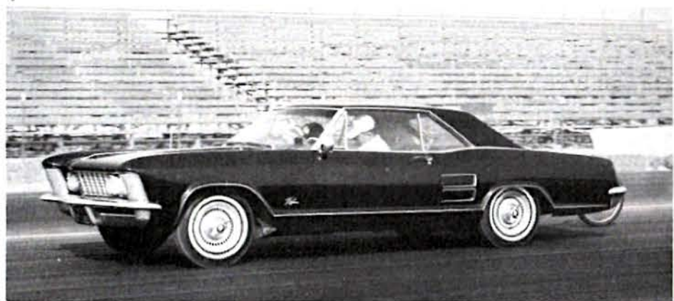
Offering the most power in the Buick line was the "new for '63" Riviera. An optional 425cid engine made 340 hp @ 6000 rpm.
