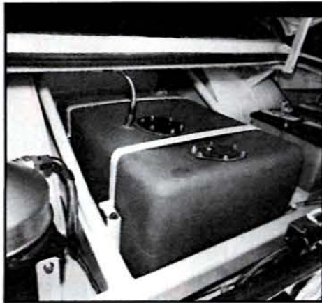
Not much room for luggage in here. Twin Delco batteries assure ease of starting, even with 510 cubic inches to spin over. The Harwood fuel cell features special internal baffling that allows accurate fuel gauge readings, while the engine's dry sump reservoir also includes a handy dipstick to check the oil level.
