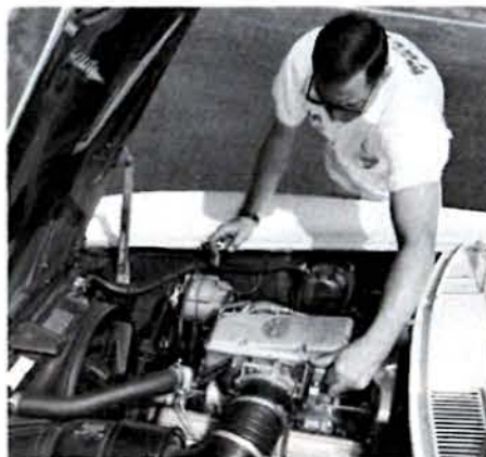
Along with a totally redesigned body and independent rear suspension, the Corvette also received a top-of-the-line, 360-horse injected 327.
