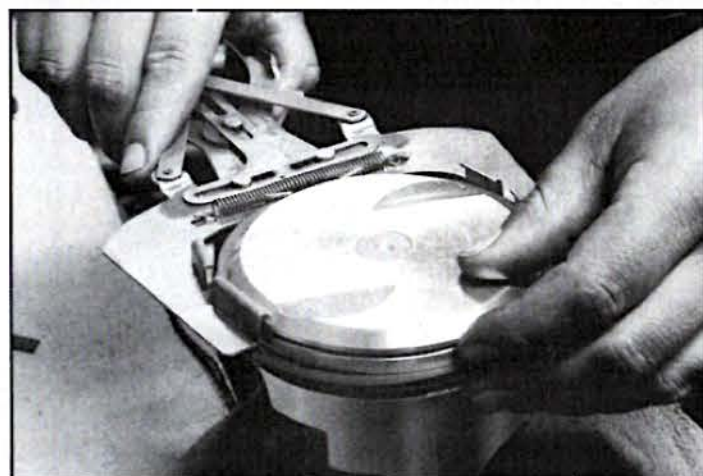
TRW .030-over pistons (TRW L2377F) were fitted with TRW ceramic-coated rings because of their resistance to the side effects of detonation. Stock 454 rods were fitted with Specialty Fasteners' high-strength rod bolts, but only after the rods were checked for straightness and resized on both ends.
