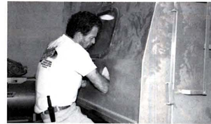
The secret to powder adhesion is a well-prepared surface, which Dick thoroughly cleans by sandblasting.
