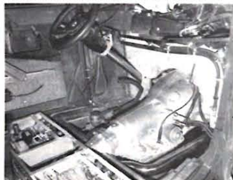
Here you can see the electronics under the front seats, as well as the air conditioning system that will be hidden in the cowl area.
