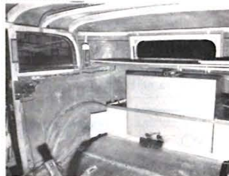
Just below the quarter window sill is the keyless entry control which is connected to the solenoid in the door jamb. Also visible prior to upholstery are the gas tank, battery box and tool storage.
