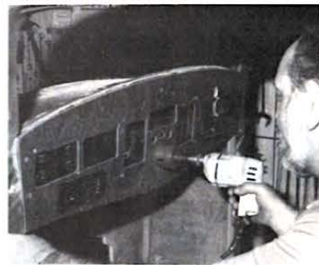
To locate our Corvette dash displays, Carl Sulkey cut out this masonite mock-up panel. Dan Fink used it as a pattern for the steel dash he made.
