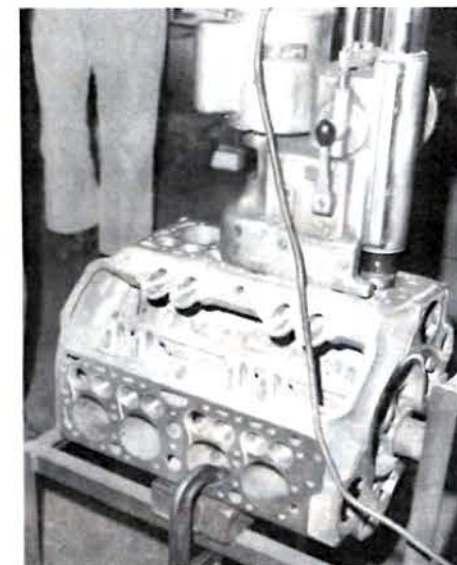
The cylinder-boring machine (called a boring bar) is clamped on the block, usually over the cylinder that is worn the most to ensure that it will clean up and accept the next larger oversize piston.
