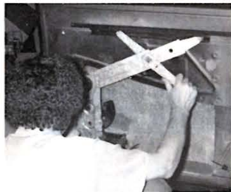
Paul Rick cut the dark-tinted glass to fit our chopped window frames and installed GM/power window lifts in the doors.
