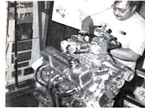
Blower Drive Service came over to check out our supercharger installation, and stayed long enough to bend some stainless steel spark plug wire conduits.
