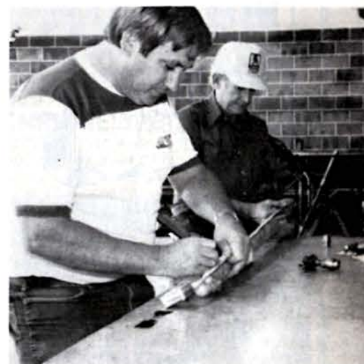
Eddie (left) and right hand man (on Eddie's left) Marvin Shaffer, measure a split-wishbone radius rod, preparing to cut the end and insert a threaded bung.
