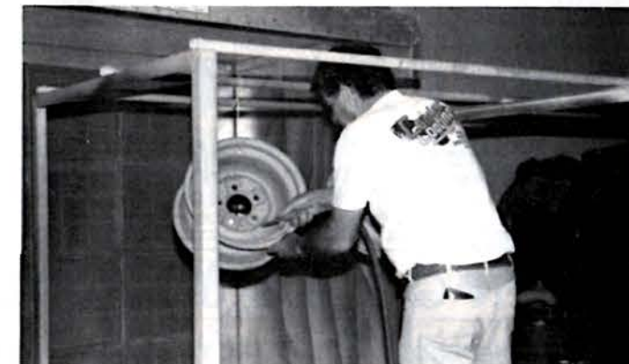
ABOVE AND BELOW — Dick hangs the wheels on the rack, making a final, essential leftover check for any sand or dust particles.
