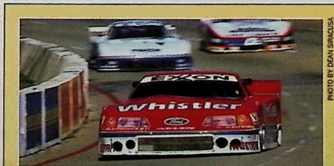
■ Robbie Gordon's banged-up but durable new Roush IMSA GTD Mustang, with square-tube frame, rear transaxle, lots of Kevlar and carbon fiber and 650 turbocharged horsepower, finished 2nd to Steve Millen's Nissan at Long Beach.
