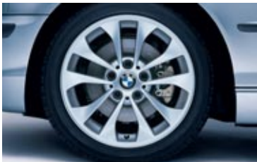
17 x 70 Double Spoke (Styling 98) alloy wheels and 205/50R-17 run-flat all-season tires can operate even when punctured, for a distance of up to 100 miles. Comes with Flat Tire Warning; space-saver spare replaces full-use spare and wheel.
