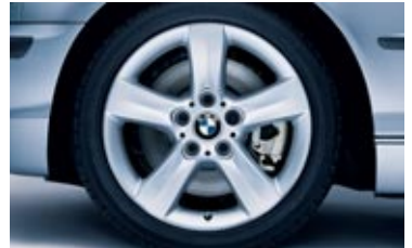
17 x 8.0 Star Spoke (Styling 119) alloy wheels and 225/45R-17 performance tires 1 make the most of the sport suspension.
