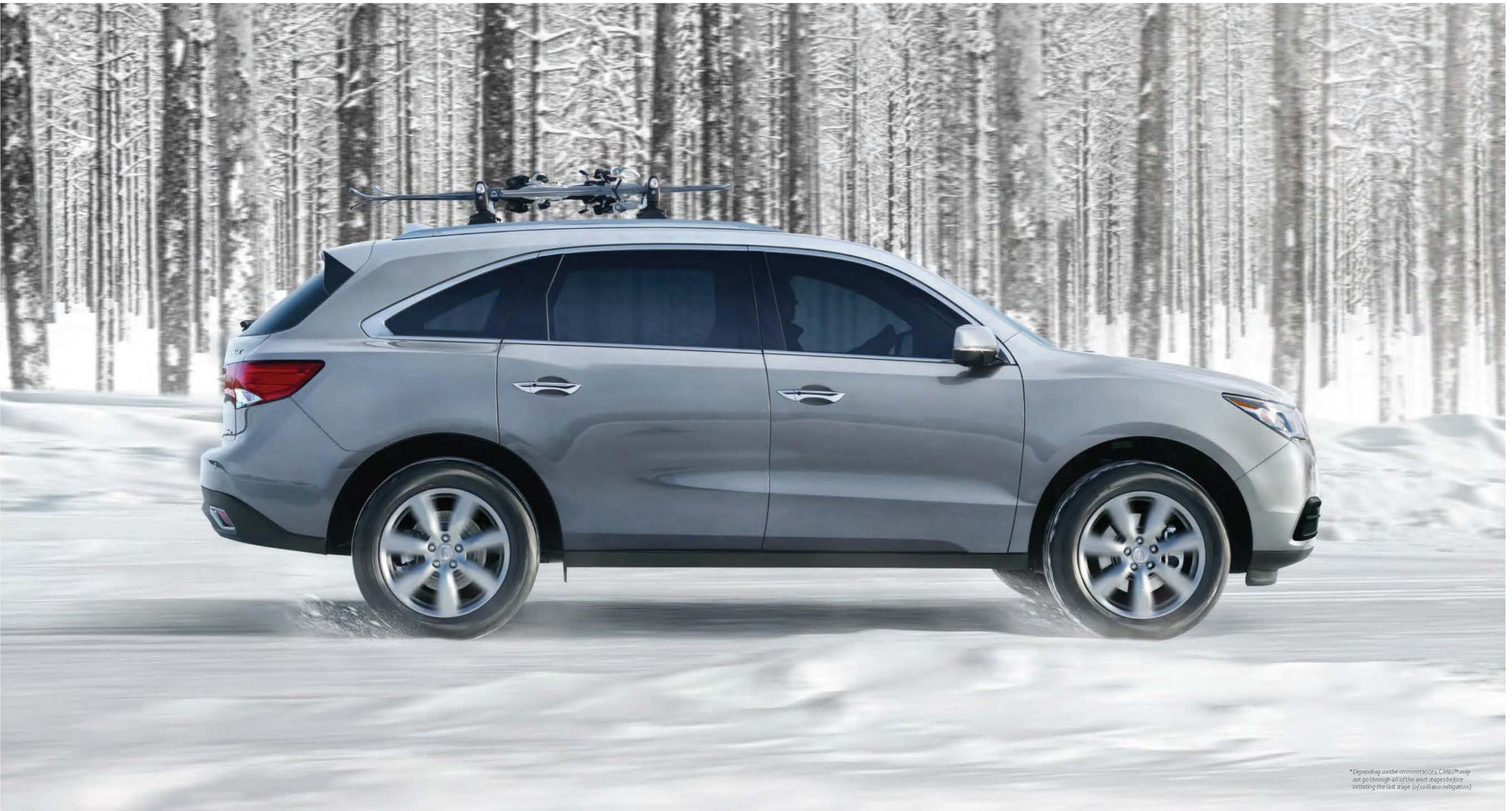
The best way to deal with a collision is to never have one. Fortunately, the new MDX has numerous features that work in concert to help keep you on your intended path through poor weather or on rough, slippery roads. SH-AWD partners with Vehicle Stability Assist™ (VSA®) to limit wheel spin and send power to those wheels with the most traction.
