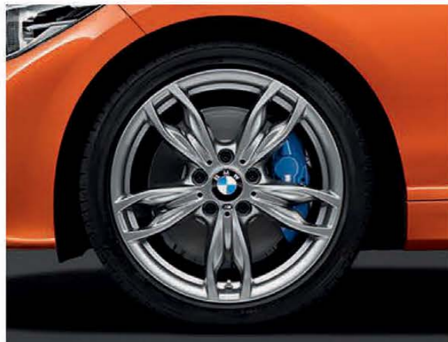
18" M light alloy wheels Double-spoke style 436 M with mixed tyres, front 7.5 J x 18 with 225/40 R 18 tyres, rear 8 J x 18 with 245/35 R 18 tyres.
