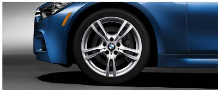
Star Spoke light alloy wheels (Style 400M) . With run-flat 1 all-season tires 2 : 18 x 8.0 and 225/45 tires. With run-flat 1 performance tires 2,3 : 18 x 8.0 front, 18 x 8.5 rear and 225/45 front, 255/40 rear tires (includes increased top-speed limiter).
