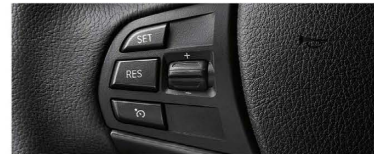
Dynamic Cruise Control 4 lets you set and keep to a chosen speed above 20 mph, including automatic application of the brakes when driving downhill. It is activated and regulated via controls positioned on the left side of the steering wheel, and deactivated by applying the brakes or switching off the feature.
