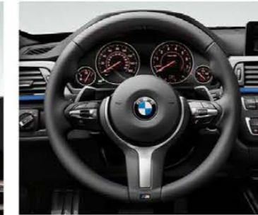
Three-spoke, leather-wrapped multi-function M sport steering wheel includes a thick, textured rim and thumb indents that are designed for performance driving. Multi-function buttons let you adjust various comfort features while keeping both hands on the wheel.
