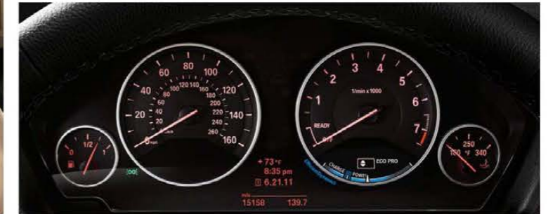
Instrument panel features a red backlit speedometer and tachometer. Centered between the two easy-to-read analog instruments is the on-board computer with liquid crystal display providing additional important driving information. Extended instrument cluster , included with the Navigation system, has a high-resolution Info Display showing functions for the Check Control as well as Navigation system prompts and operational feedback. With the ECO PRO mode activated, EfficientDynamics information is displayed in the rev counter.
