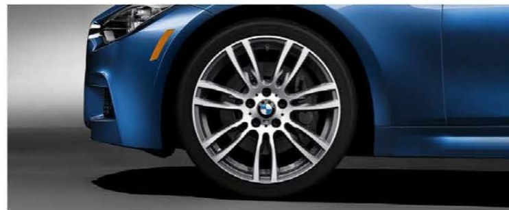
Star Spoke light alloy wheels (Style 403M) with 19 x 8.0 front, 19 x 8.5 rear and 225/40 front, 255/35 rear run-flat 1 performance tires 2,3 (includes increased top-speed limiter).
