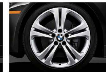
Double Spoke light alloy wheels (Style 401) with 19 x 8.0 front, 19 x 8.5 rear and 225/40 front, 255/35 rear run-flat 1 performance tires. 2,3 (Includes increased top-speed limiter.)
