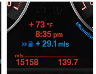
On-board computer provides data on exterior temperature, average speed, average and current fuel consumption, and range. With the ECO PRO mode activated, the current bonus range is also displayed.
