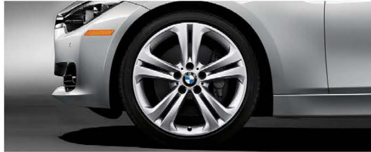
Double Spoke light alloy wheels (Style 401) with 19 x 8.0 front, 19 x 8.5 rear and 225/40 front, 255/35 rear run-flat 1 performance tires 2,3 (includes increased top-speed limiter).
