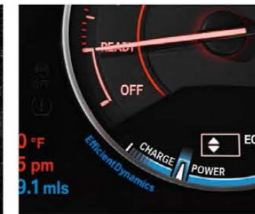
Auto Start-Stop function switches off the engine automatically during brief stops, such as at red lights, to reduce fuel consumption. A symbol displayed in the rev counter indicates that the function is active.
