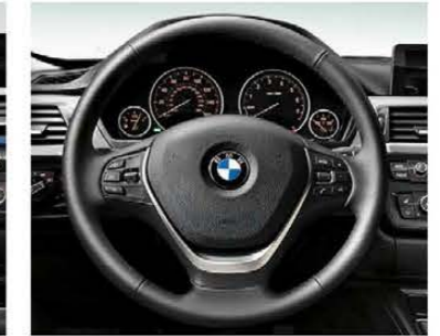
Three-spoke leather-wrapped multi-function steering wheel provides buttons on the left for operating the cruise control functions; buttons on the right adjust all audio-related functions, including Bluetooth enabled mobile phone.
