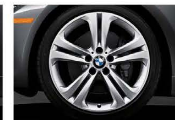
Double Spoke light alloy wheels (Style 401) with 19 x 8.0 front, 19 x 8.5 rear and 225/40 front, 255/35 rear run-flat 2 performance tires. 3,4 (Includes increased top-speed limiter.)
