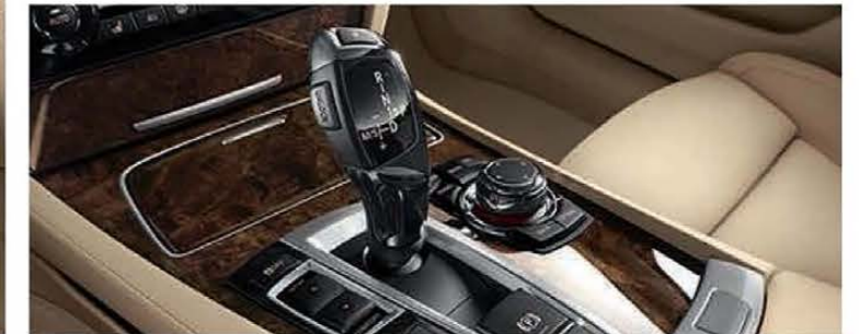
8-speed STEPTRONIC automatic transmission with Adaptive Transmission Control (ATC) provides extremely fast synchronized shifting in either the Sport or Manual shift mode. By increasing the number of gears to eight, the transmission provides a more efficient shifting sequence and improved fuel economy.
