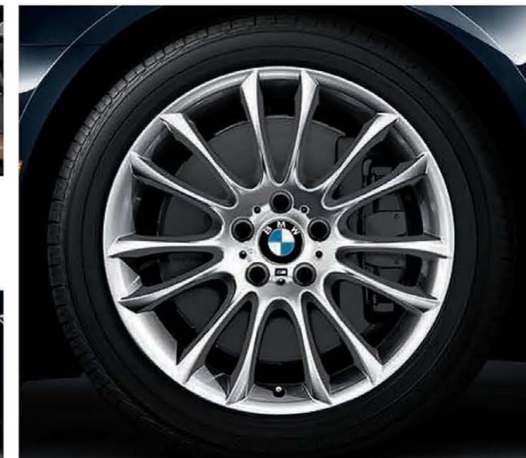
V Spoke (Style 302M) M light alloy wheels, 19 x 8.5 front, 19 x 9.5 rear, with 245/45 front, 275/40 rear run-flat 1 performance tires. 2 Also available: V Spoke (Style 302M) 19 x 8.5 M light alloy wheels with 245/45 run-flat 1 all-season tires. 2
