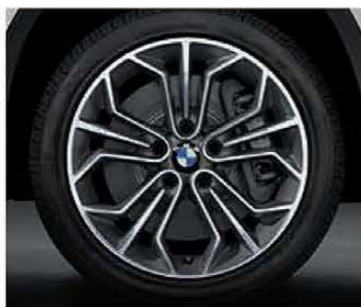
Honeycomb light alloy wheels (Style 323) , 18 x 8.0 front, 18 x 9.0 rear; and 225/45 front, 255/40 rear run-flat 1 performance tires. 2,3
