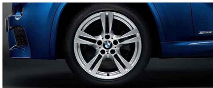
Double Spoke light alloy wheels (Style 355M) . With run-flat 1 all-season tires 2 : 18 x 8.0; and 225/45 tires. With run-flat 1 performance tires 2,3 : 18 x 8.0 front, 18 x 9.0 rear; and 225/45 front, 255/40 rear tires (includes increased top-speed limiter).
