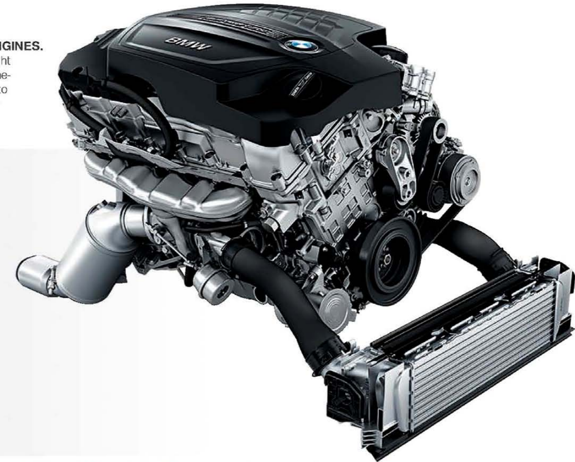
300-hp BMW TwinPower Turbo inline six-cylinder engine.
