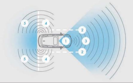
FORWARD COLLISION WARNING (FCW) & COLLISION MITIGATION BRAKING SYSTEM™ (CMBS) When a driver is traveling above 10 mph, Forward Collision Warning can trigger an audible alert and a visual warning on the dash if it senses there is danger of a collision with a vehicle detected ahead.\* If the driver does not slow down and the system still senses the driver is at risk, CMBS™ can brake lightly and tug at the driver's seatbelt. In a final effort to avoid or decrease the likelihood of a collision.
