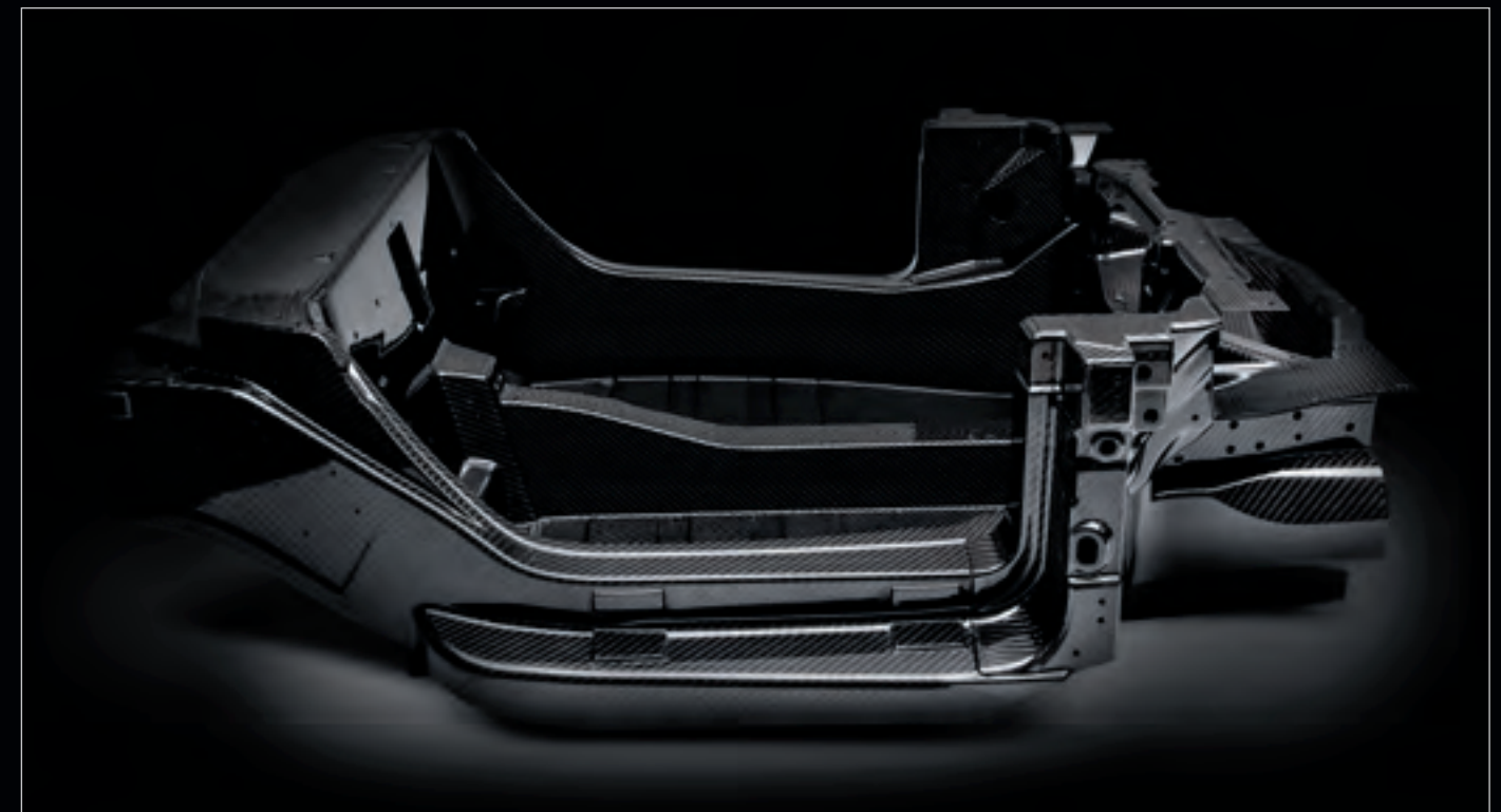
Genuine carbon fiber monocoque chassis
