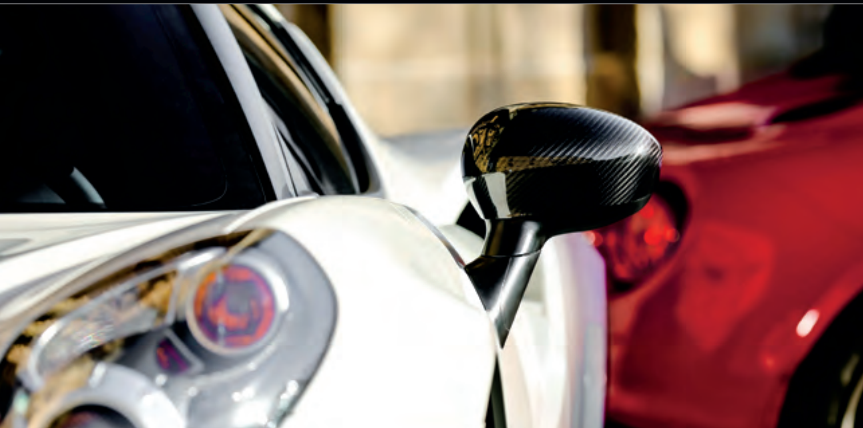
Handcrafted in Modena, Italy, each 4C model features interior and exterior design elements that conspire to win you over, channeling the unique Alfa Romeo spirit. Ultralight and strong, carbon fiber is a key structural component as well as a distinctive embellishment, including the all-new carbon fiber roof, and as shown above on the mirror cover.
